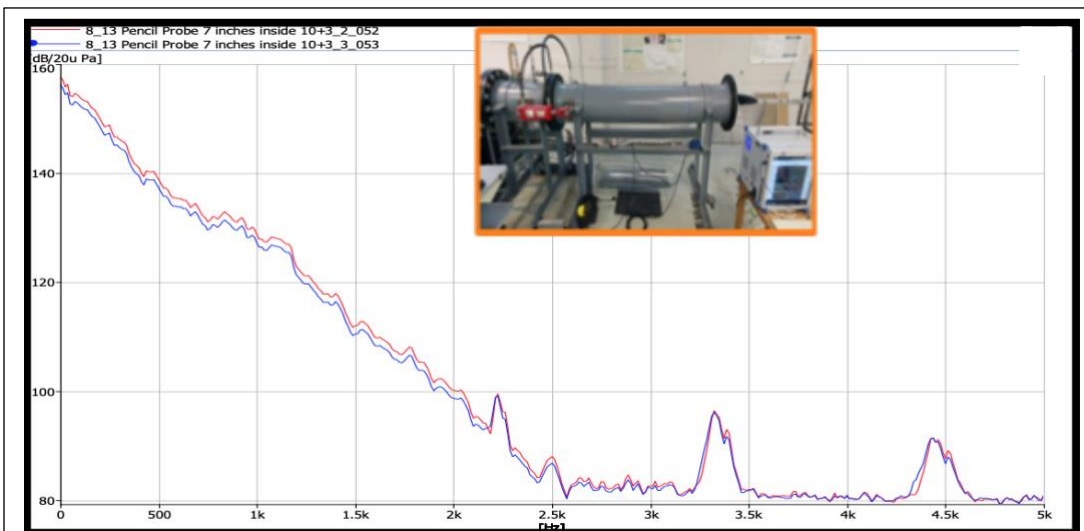
Figure 2. Shortening the length of the shock tube leads to sound pressure levels extending over wider frequencies at higher intensities.
