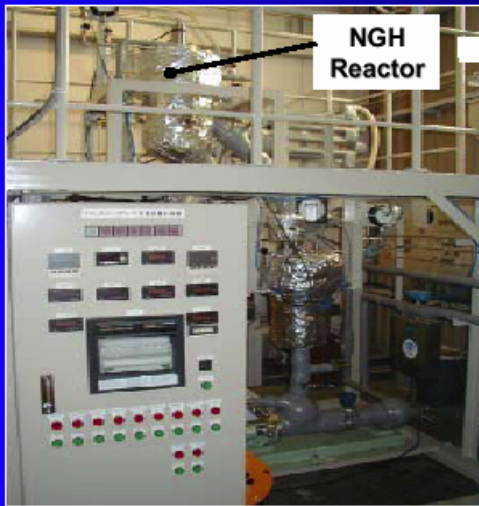
Bench Scale NGH Production Equipment (Capacity is about 5kg NGH per hour) in Mitsui's Chiba Laboratory
