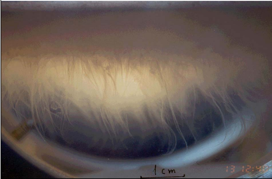
Natural gas Hydrate crystals formed in Water+Kinetic Inhibitor
