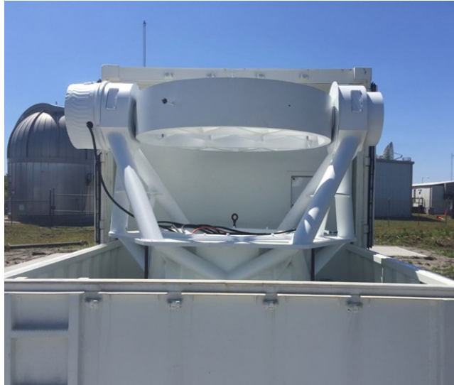
Figure 5: The LOTIS optical tracker installed in the MU-HELF.
