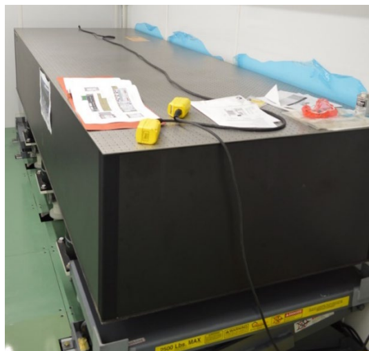
Figure 3: The optical table as installed in the MU-HELF cleanroom. Photo taken upon container delivery, thus packing materials are still visible on the walls.
