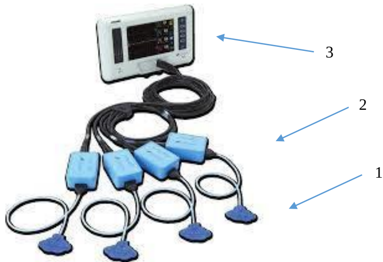
Figure 4. The NONIN Equanox Model 7600 regional oximeter system consisting of: 1. adhesive patches containing the IR source and sensor matrix; 2. signal processing unit; 3. display monitor containing the data acquisition system.
