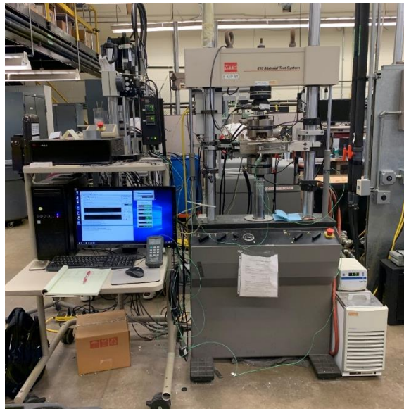
Figure 3. Test Station with 5-kip MTS and accompanying equipment
