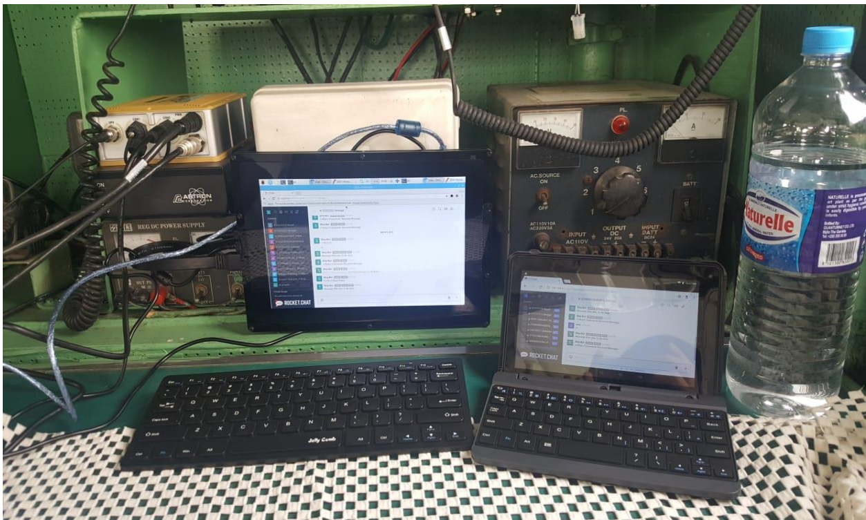
Figure 3. Chat-over-AIS installed on GAB Musamaliya vessel.
