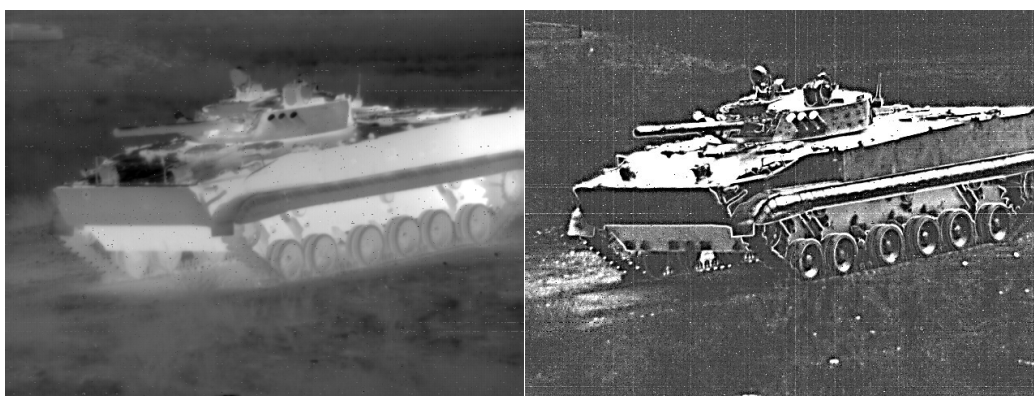
Fig. 2 LWIR thermal (left) and polarimetric DoLP (right) image comparison of a Russian 1970s vintage T-72 tank
