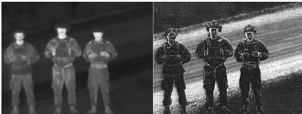
Fig. 1 LWIR thermal (left) and polarimetric DoLP (right) image comparison of Soldiers recorded at Ft Hunter Liggett
