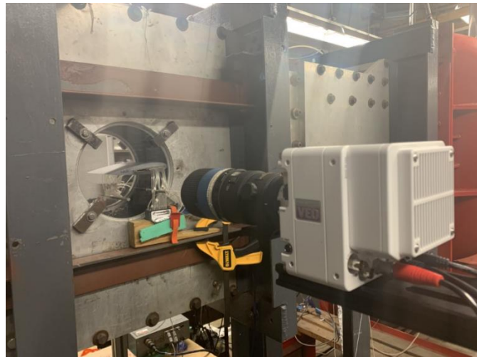
Figure 10: Experimental setup of the BOS technique for Mach oscillation measurements.
