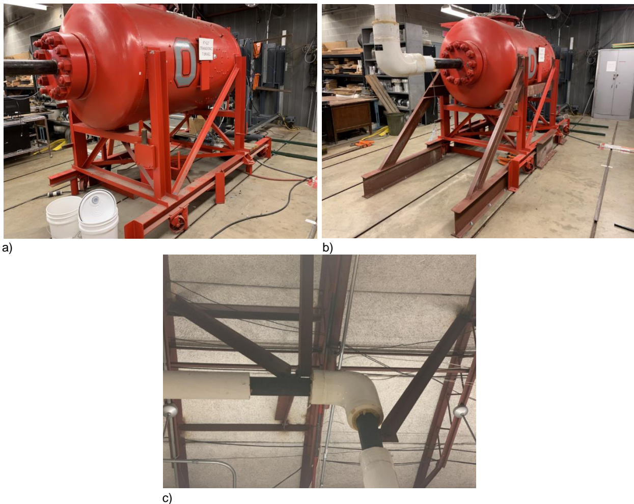
Figure 1: Structural stabilization to the wind tunnel to mitigate longitudinal vibration: a) before stabilization, b) stabilization of the settling chamber, c) stabilization of the pressurized air supply line.
