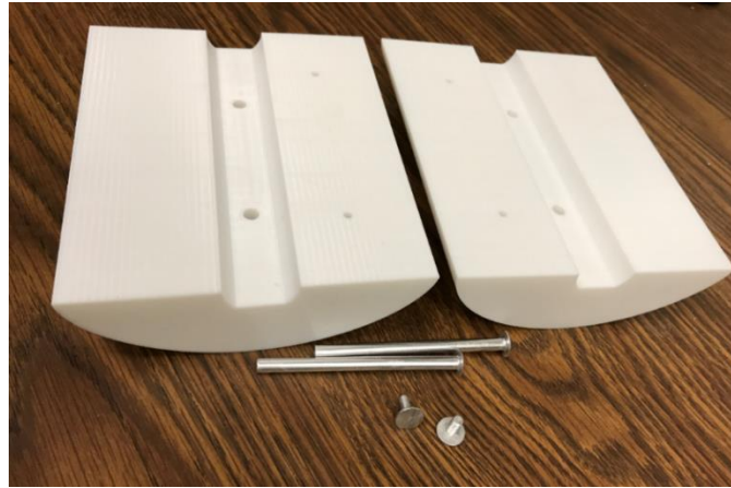
Figure 4: 3D printed elliptical choke vane for Mach oscillation.
