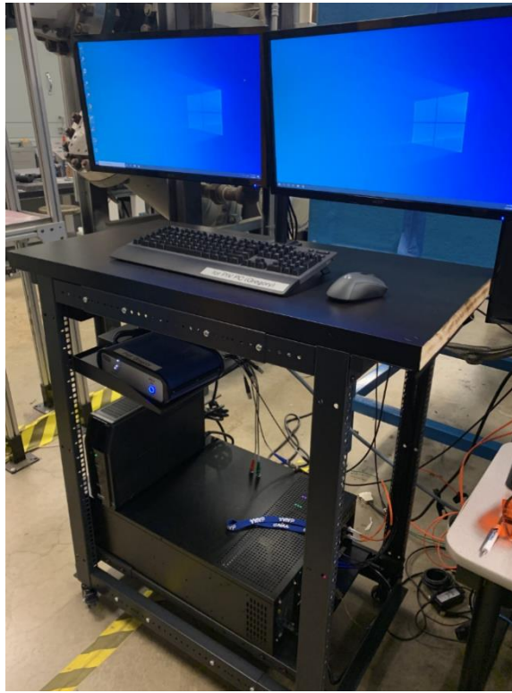
Figure 8: PIV system upgrade components: a) upgraded duo sCMOS cameras, two on the left. b) upgraded optical data processing workstation, include upgraded DaVis software, GPU processing capability, upgraded PTU, etc.
