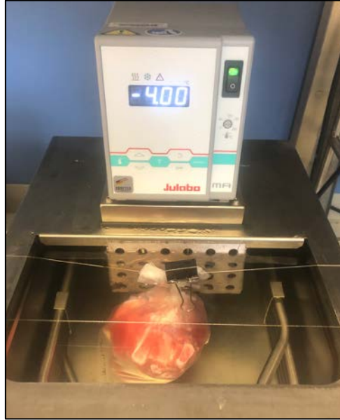
Figure 6. VCA supercooling. Swine partial hind limb stored in a sterile bag in HTK. Chiller set at -4^{\circ}\text{C} .
