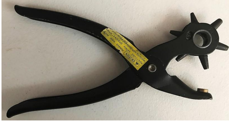
Fig. 4 Leather punch used for making holes in the vinyl
