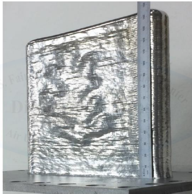
Figure 6: Oak Leaf image in titanium wall build resulting from melt pool size control 61
