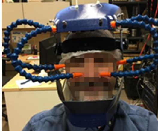
Figure 22. An example of a custom helmet with movable arms used to present short duration puffs of medical-grade nitrogen to areas on the face.
