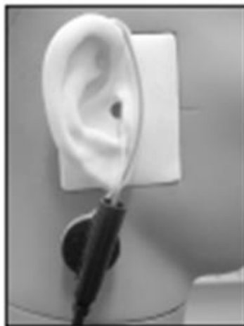
Figure 21. Etymotic Research ER7C probe microphone used to determine the sound field to ear-drum transfer function.
