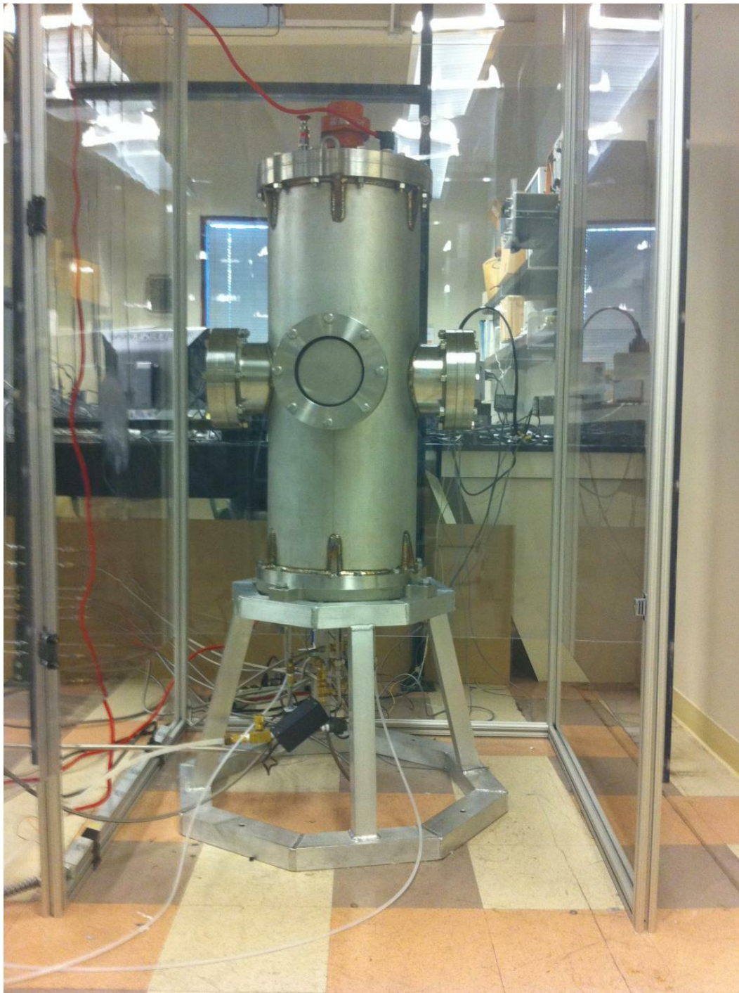
Figure 7: Photo of the stainless steel pressure chamber mounted to an aluminum stand. Flanges connecting the cylindrical part to bottom and top are reinforced with gussets. All gas lines enter the chamber through the bottom part. Top and cylindrical part of the chamber can therefore be lifted off without dismantling any connections. The chamber is enclosed in a high-impact polycarbonate cubicle that provides an increased degree of safety in case of malfunction or accident.
