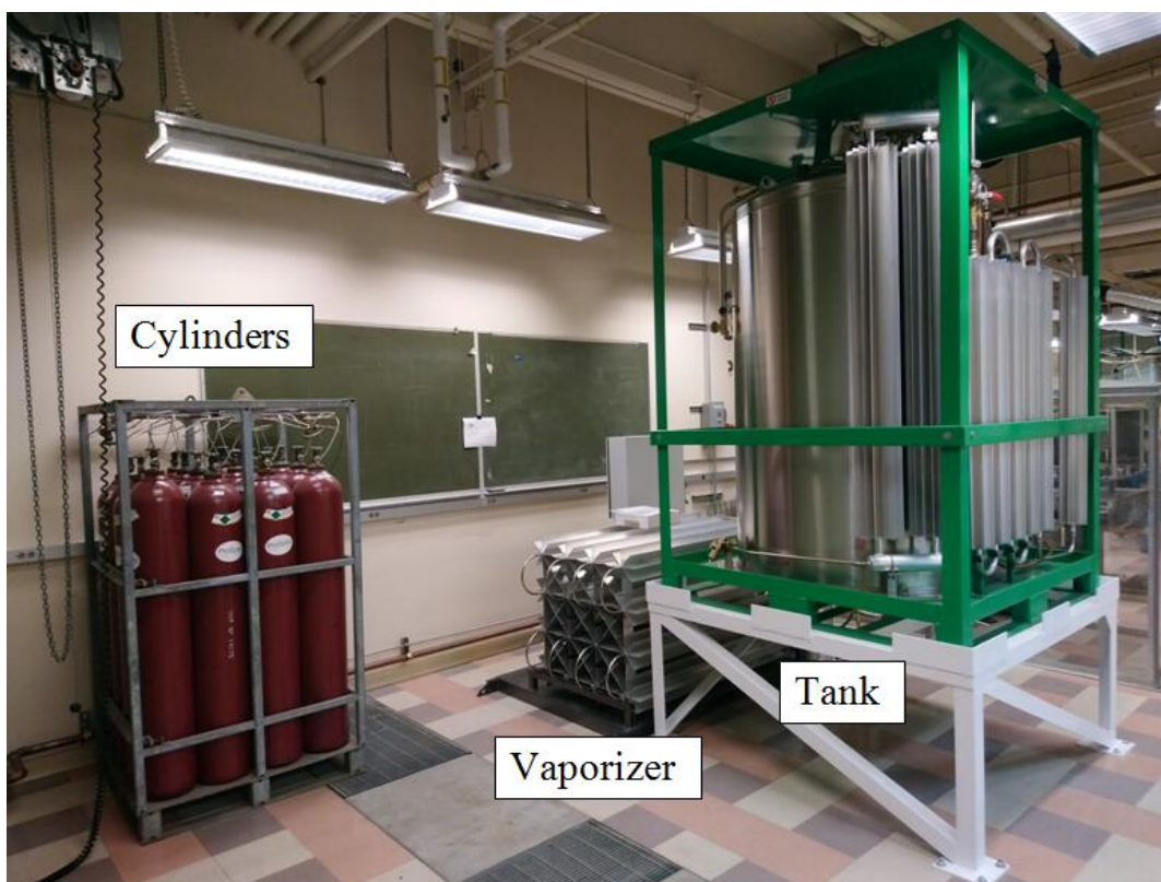
Figure 3: Photograph of the high-capacity gas-handling system. The photograph shows the liquid nitrogen tank and the 12-cylinder buffer pack
