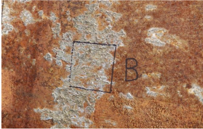
Figure 12. Photograph of Sample B before cutting from region with resolidified metal splatters.
