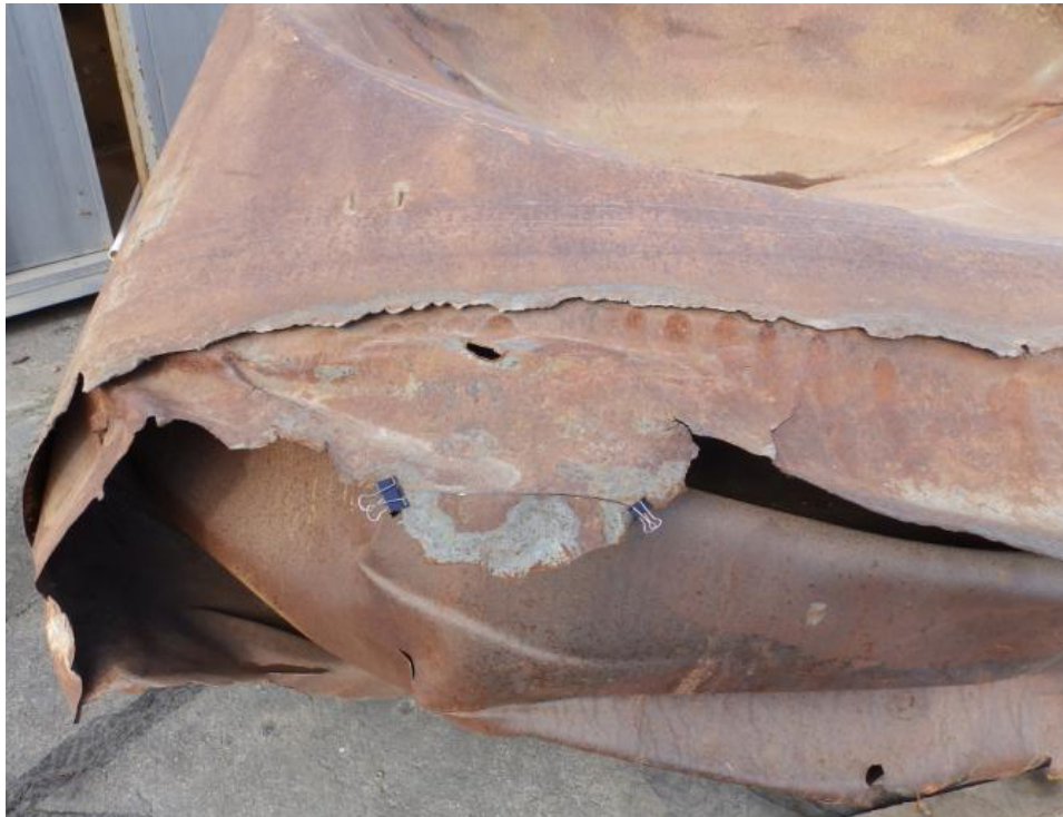
Figure 19. Photograph of Sample A1 secured to aft dome by binder clips after removal from Mongolia tank.
