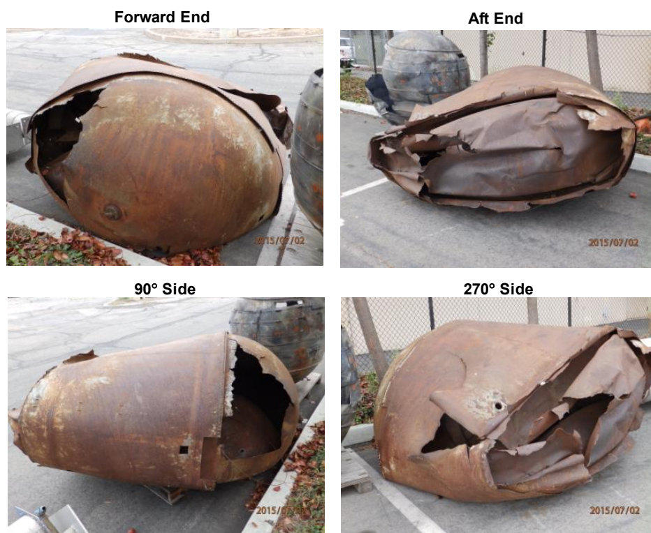
Figure 5. Photographs of Mongolia propellant tank with concave side facing downward.
