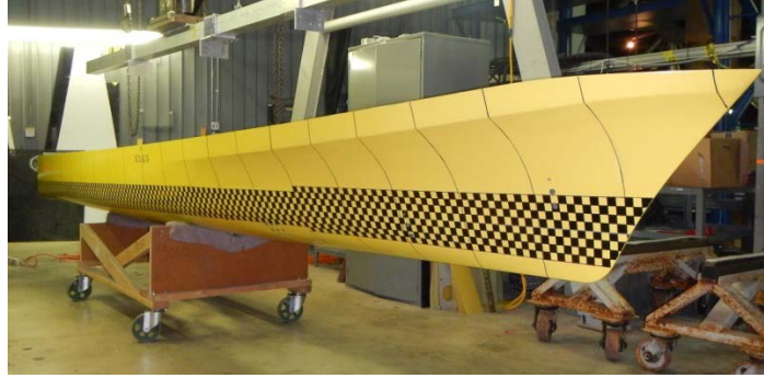
Figure 3. Image of Model 5365 showing the yellow and black paint scheme, waterlines, and station lines.
