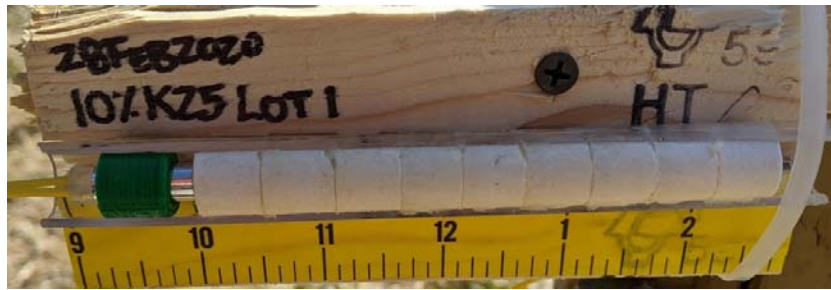
Figure 15: Shot fixture with detonator
