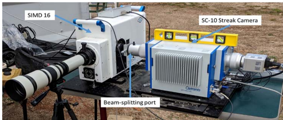
Figure 16: high-speed camera set-up
