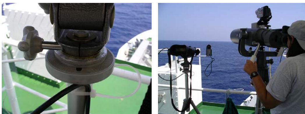
Figure 7 Particular of the tripod showing the bearing scale (left) used to point the devices to the direction detected through the long range binoculars (right).
