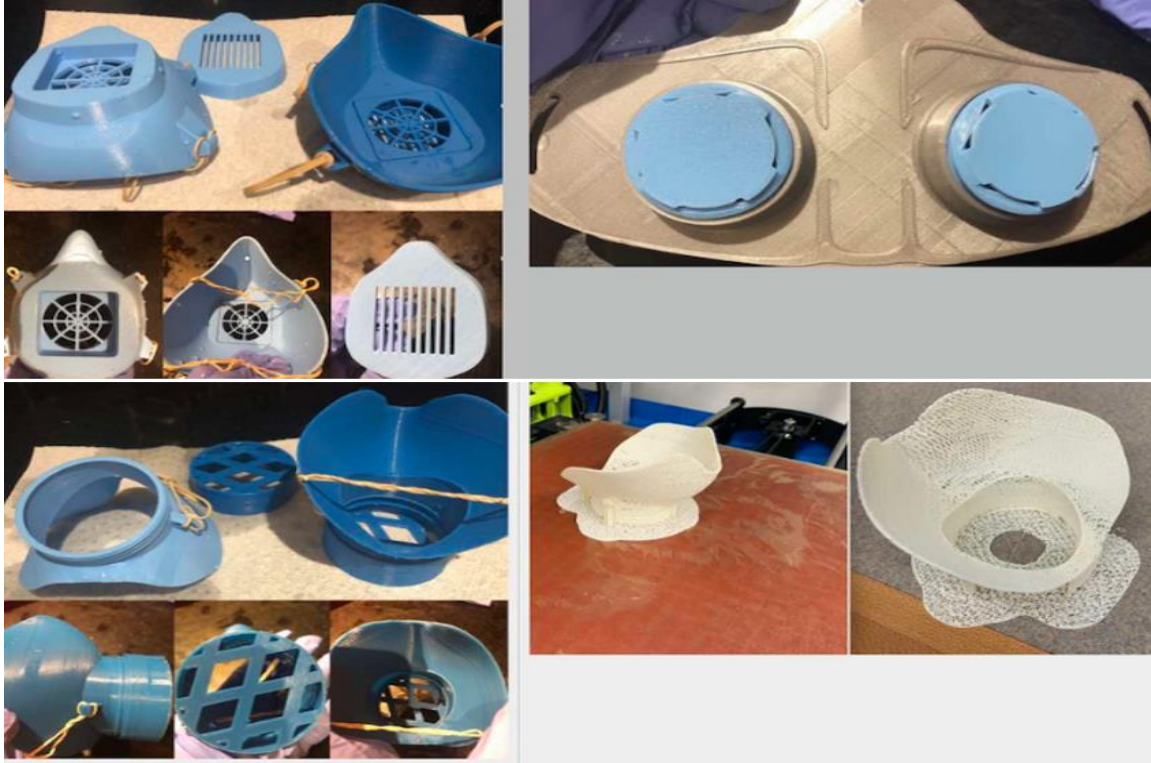
Figure 2. Making N95 Mask Using 3D Printing Technology by (GWUH) (Ms et al., 2020)
