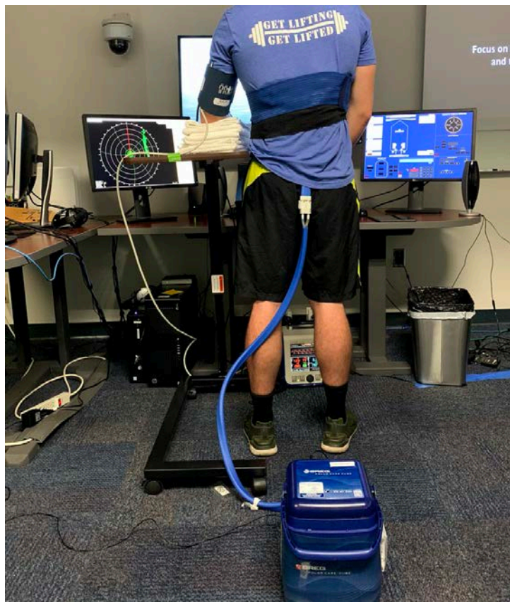
Figure 10. BREG Polar Care Cube (CWPS) Applied to Participant's Lower Back
