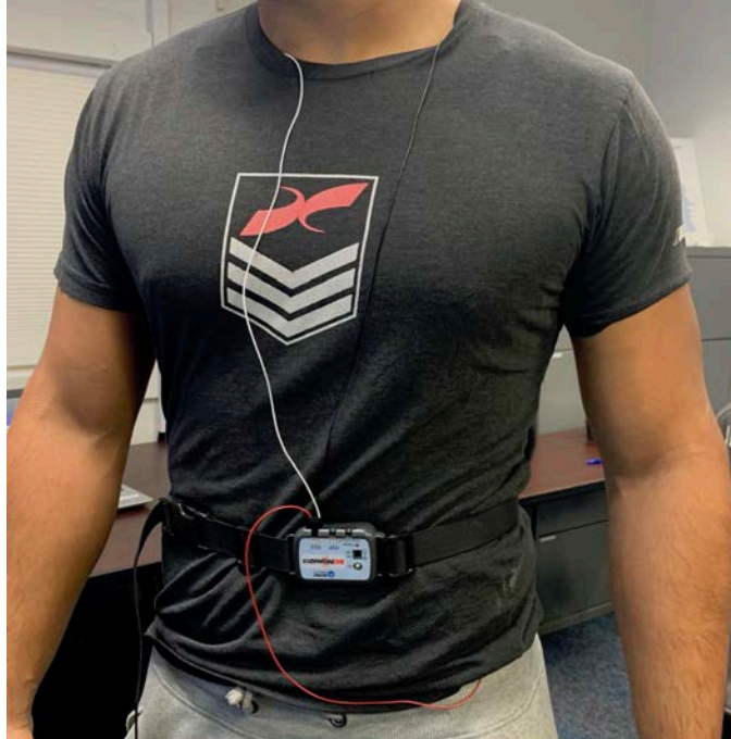
Figure 4. ECG Transmitter and Electrode Placement
