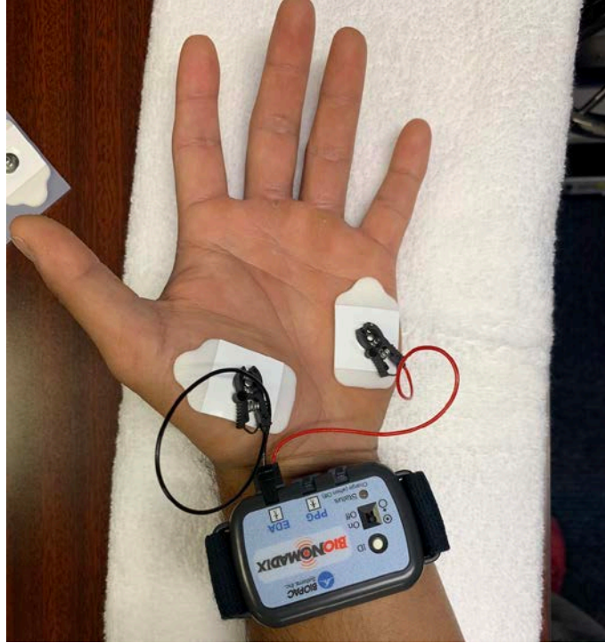
Figure 3. EDA Transmitter and Electrode Placement
