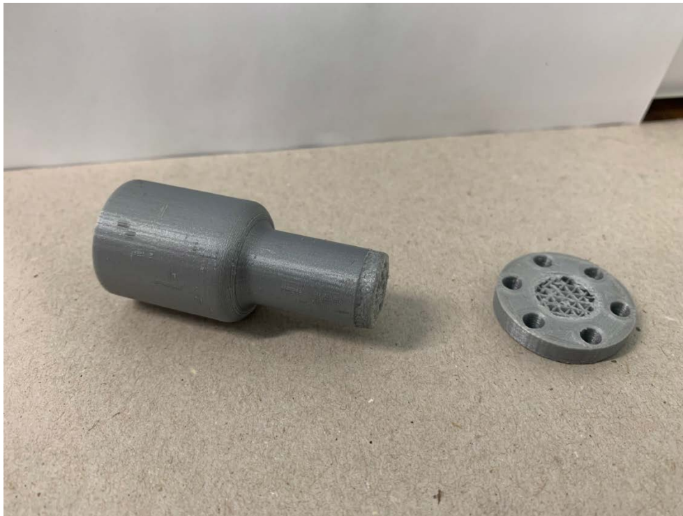
Figure 21. Failed PLA Coupling Device
