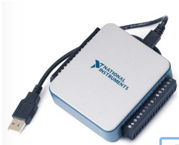
Figure 16. National Instruments Multifunction DAQ, Model USB-6003 16 Bit. Source: [9].
