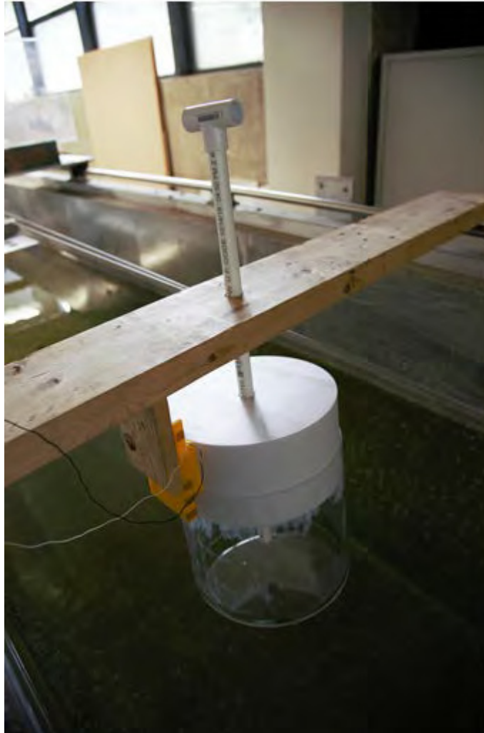
Figure 32. Final assembly of initial NPS TENG model. Source [9].
