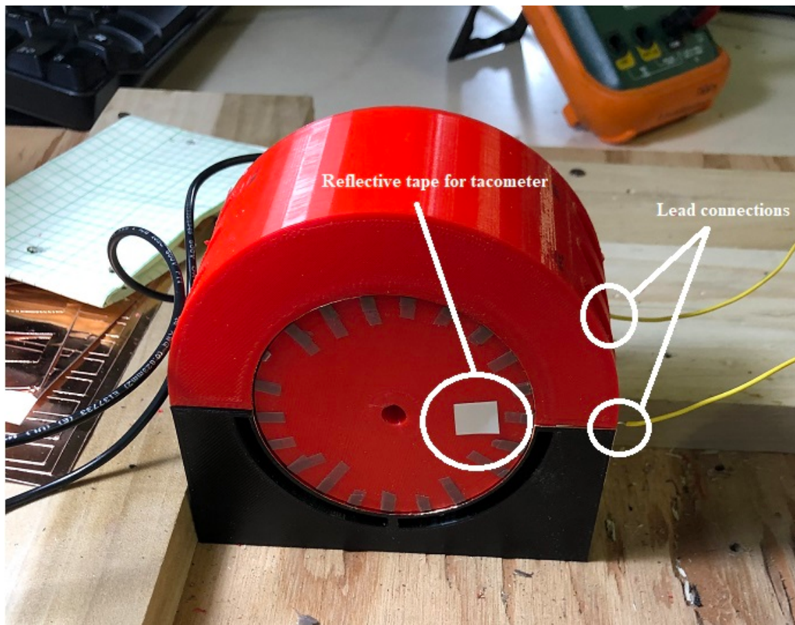
Figure 37. TENG assembly with wires attached to electrodes. and reflective tape for tachometer.
