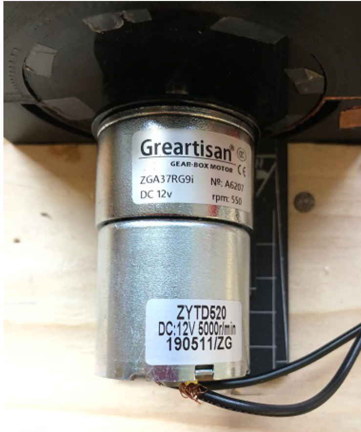
Figure 35. DC motor drives inner rod for TENG.
