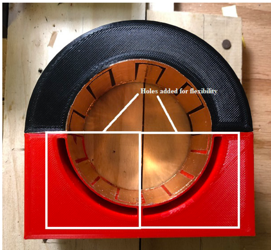
Figure 28. 3D printed assembly of final TENG design.
