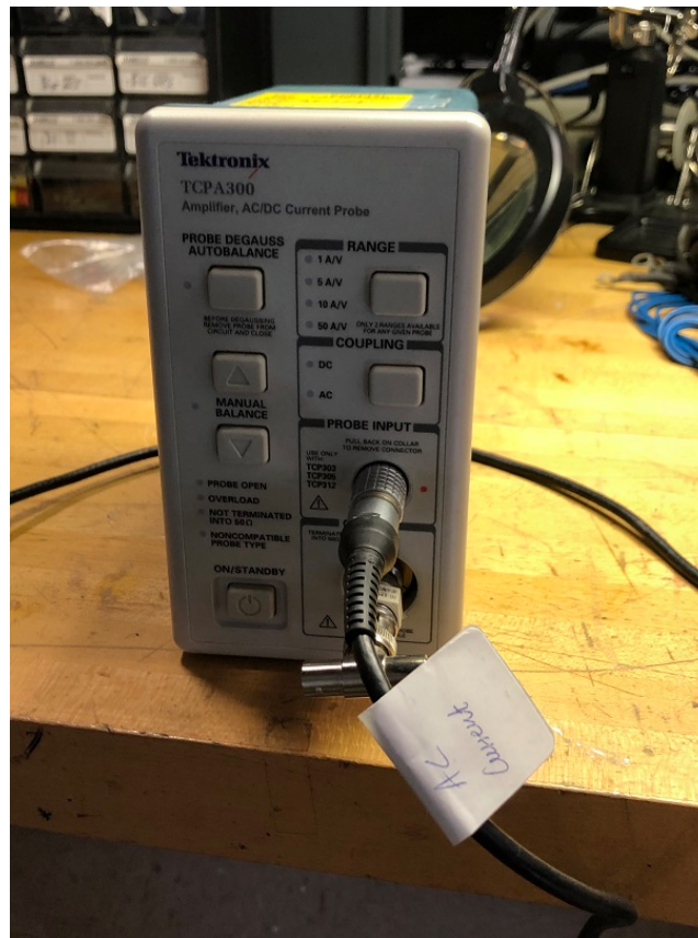
Figure 40. Tektronix TCPA300 amplifier connects to the TENG and oscilloscope.
