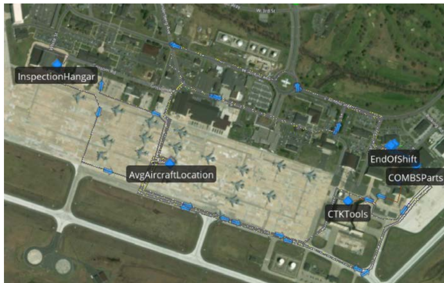
Figure 25. Aerial View of the KC-10 Simulation Workspace and the Expediter Vehicle Paths and Node Locations.
