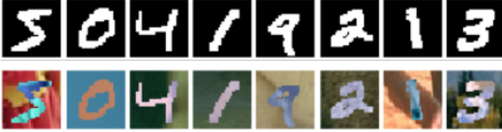
The top row of images are from the original MNIST dataset. The bottom row is the MNIST-M dataset following the transformation effected on the MNIST dataset using equation 3.18.
