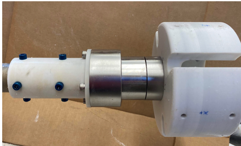
Figure 3.5. The load cell and internal connections used for the experiments.
