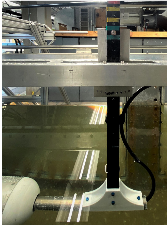
Figure 3.4. Sting and connector used to support the load cell.
