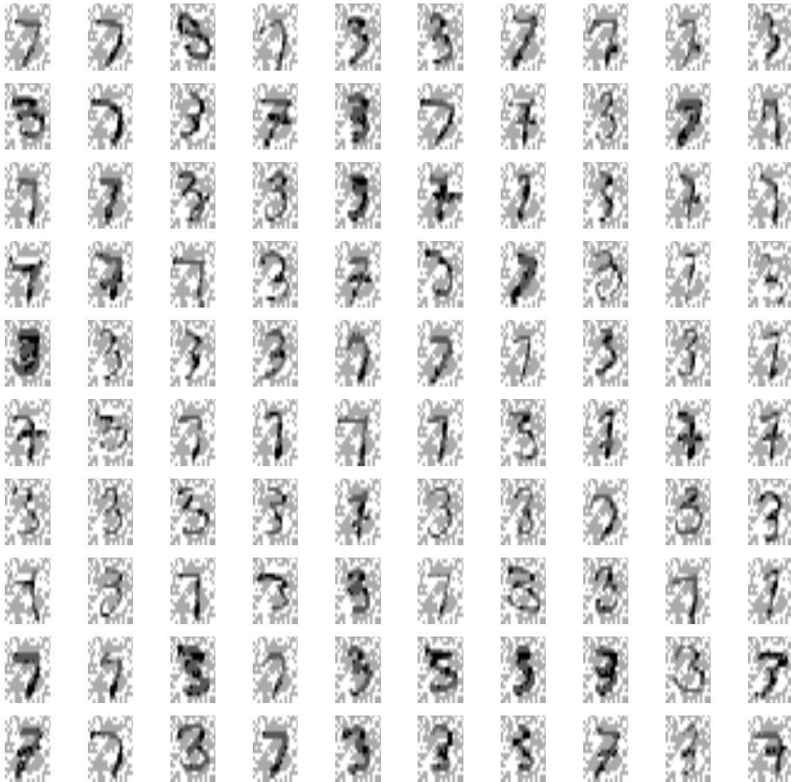
Figure 2.6. Examples of 3's and 7's in the MNIST data with FGSM perturbations.
