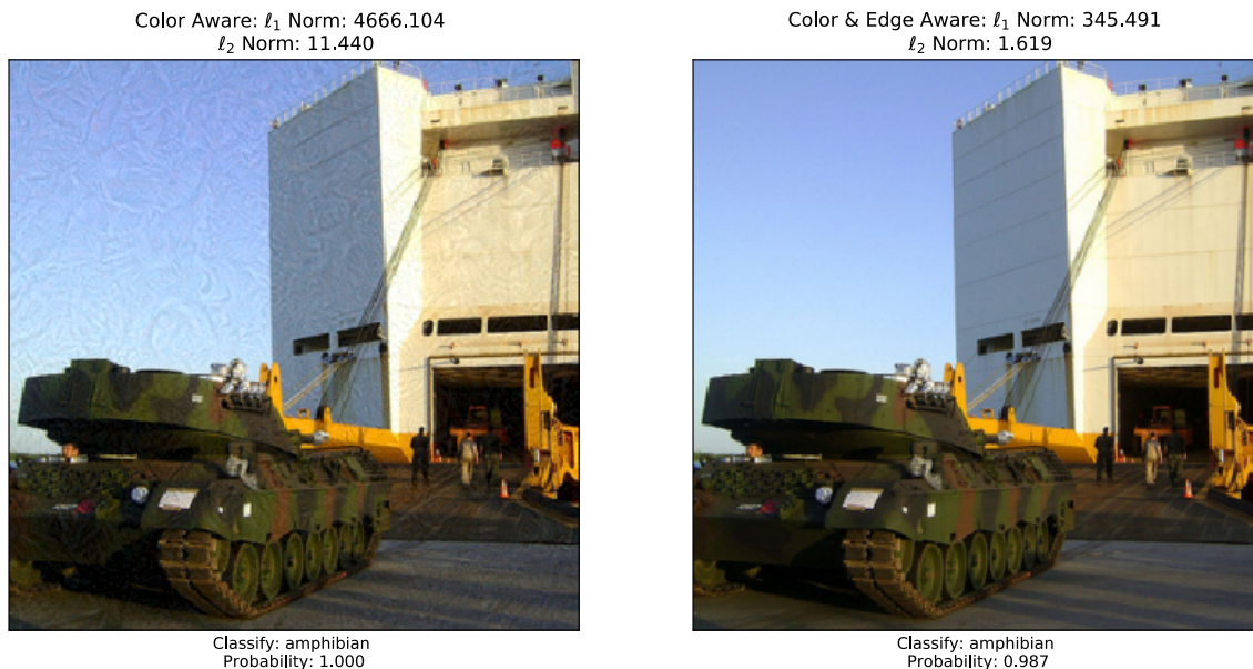
Figure 3.11. Left: Color Aware perturbation Right: Color & Edge Aware perturbation (Setting: image source - ImageNet, classifier - Inception V3, perturbation - CA and C&EA both with 6 iterations and \epsilon = 1 )
