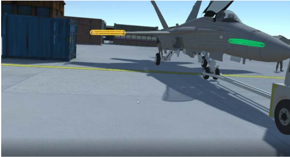
Figure 31. AR System Occluded Wingtip Visibility
