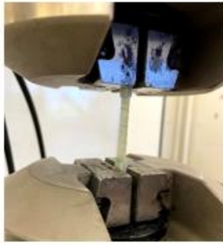
Figure 11. Setup of 0° Specimen (left) and Failure of 0° Specimen (right)
