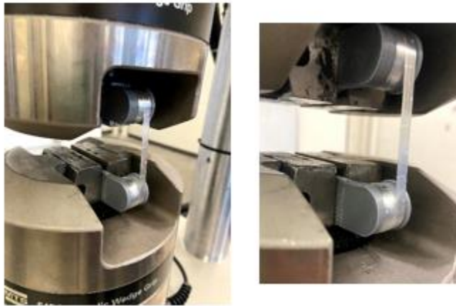
Figure 9. Setup of Fiber Bundle Fatigue Test
