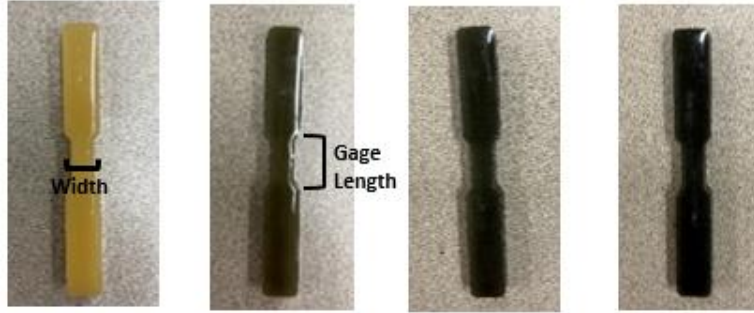
Figure 3. From left to right, Pure Epoxy, Epoxy with 0.05% CNT, Epoxy with 0.1% CNT, and Epoxy with 0.15% CNT
