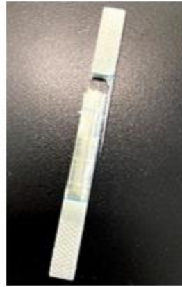
Figure 11. Setup of 0° Specimen (left) and Failure of 0° Specimen (right)
