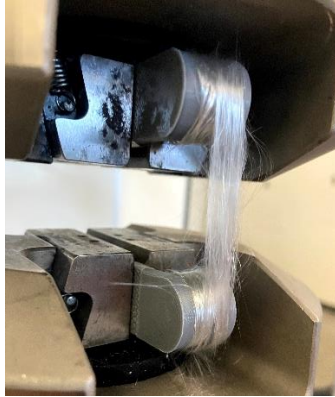
Figure 10. Failure of a Fiber Bundle at a Strain Rate of 0.07 after Approximately 160 cycles. Force Readings on the Load Cell Were below 1 N, Showing Failure of the Bundle
