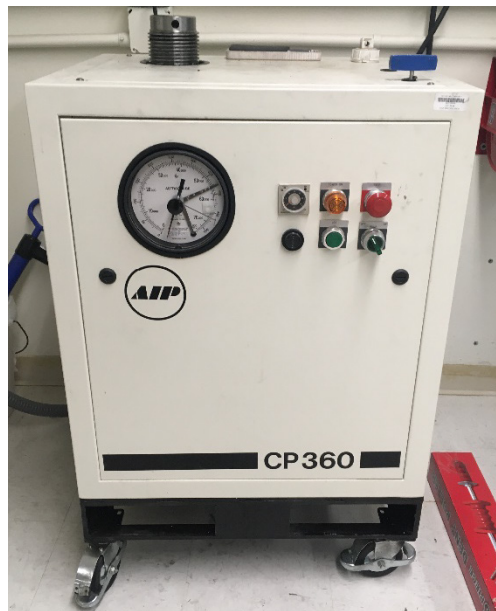
Figure 5. Cold isostatic press (CIP).
