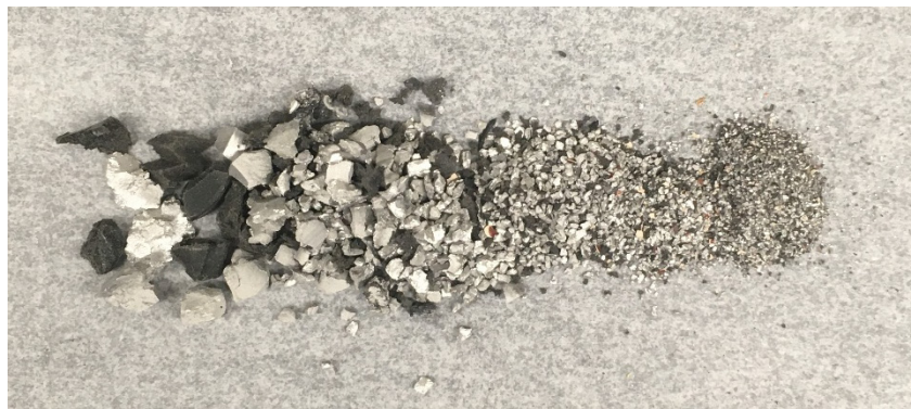
Figure 38. Fragments collected from gas gun impact.
