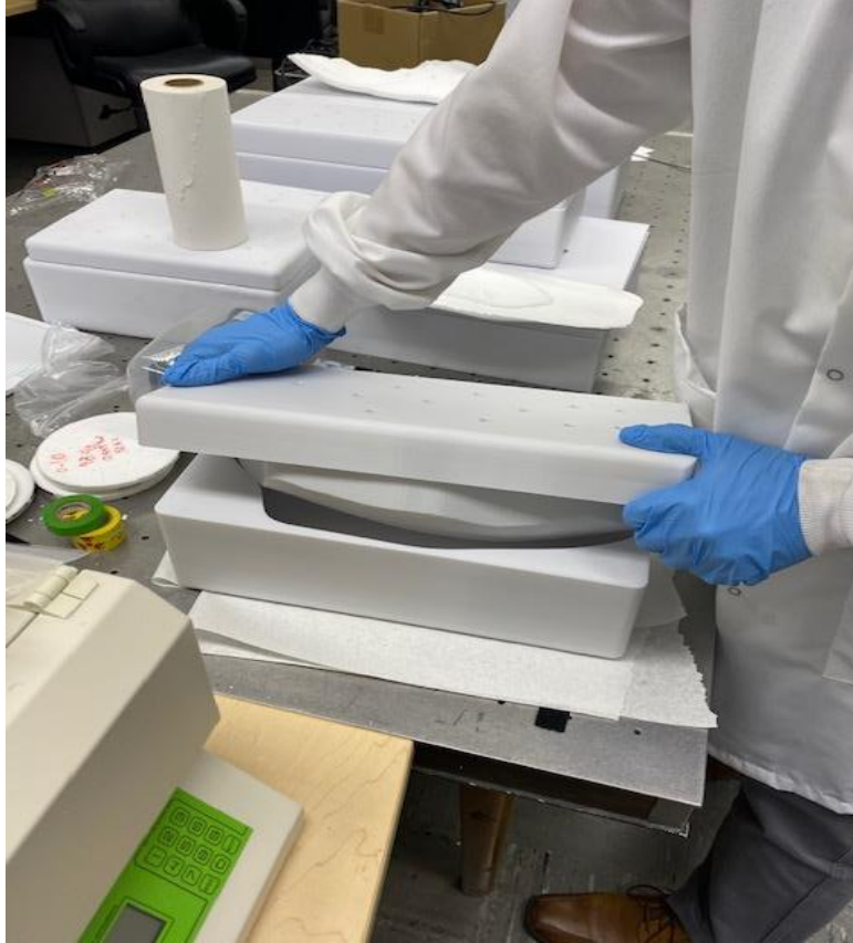
Figure 23. Mold lid is placed on bottom piece and pressed downward.
