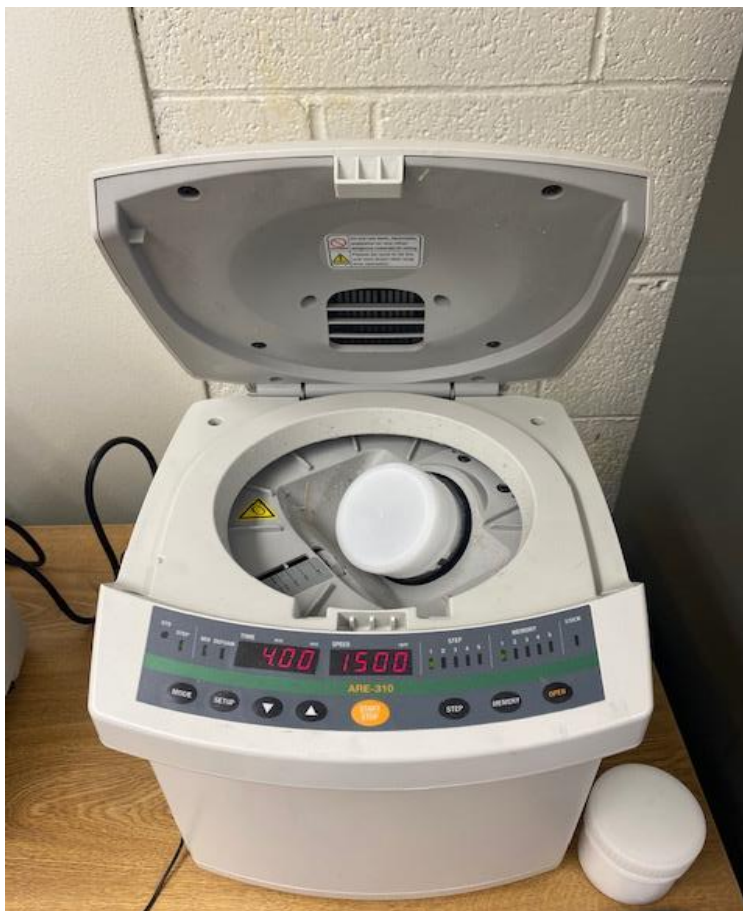
Figure 21. THINKY rotary mixer with jar inserted and times/RPMs set.
