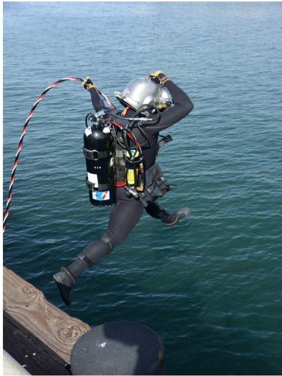
Figure 6. Diver enters the water with a hot water suit connected to surface vessel. Source: [15].
