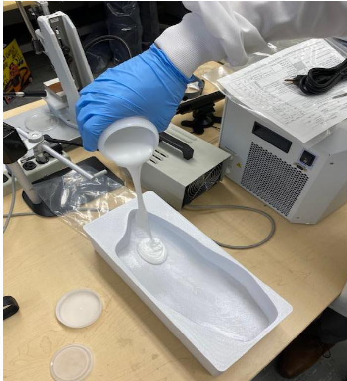
Figure 22. Liquid Composite is poured into the bottom piece of a mold.
