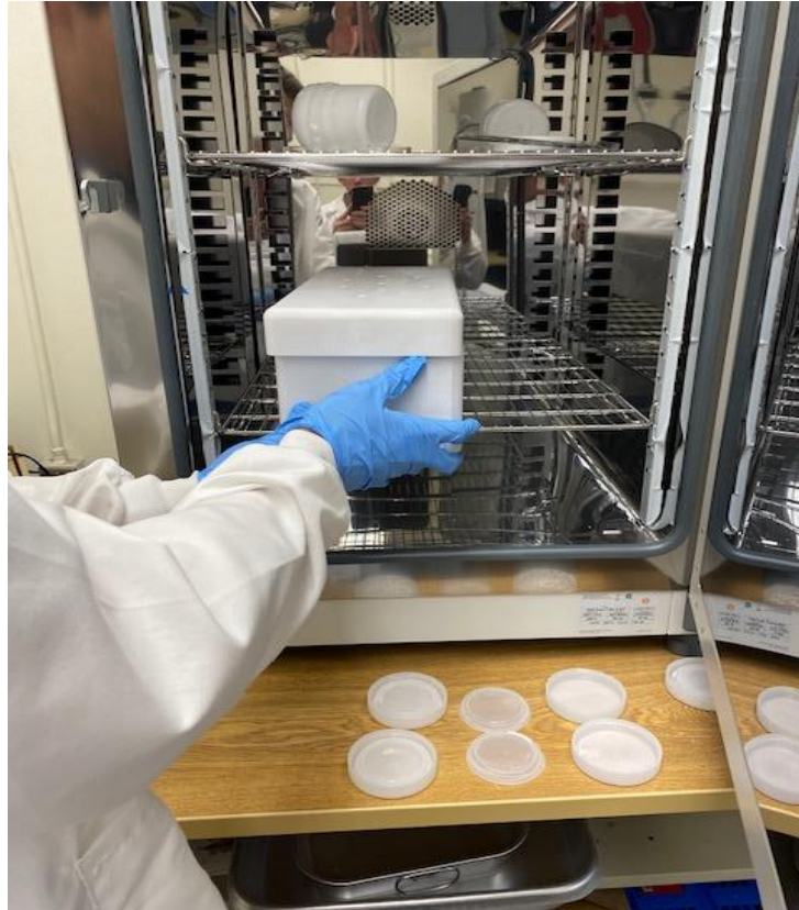
Figure 24. Mold is placed in VWR Forced Air Oven at 80 degrees Celsius.
