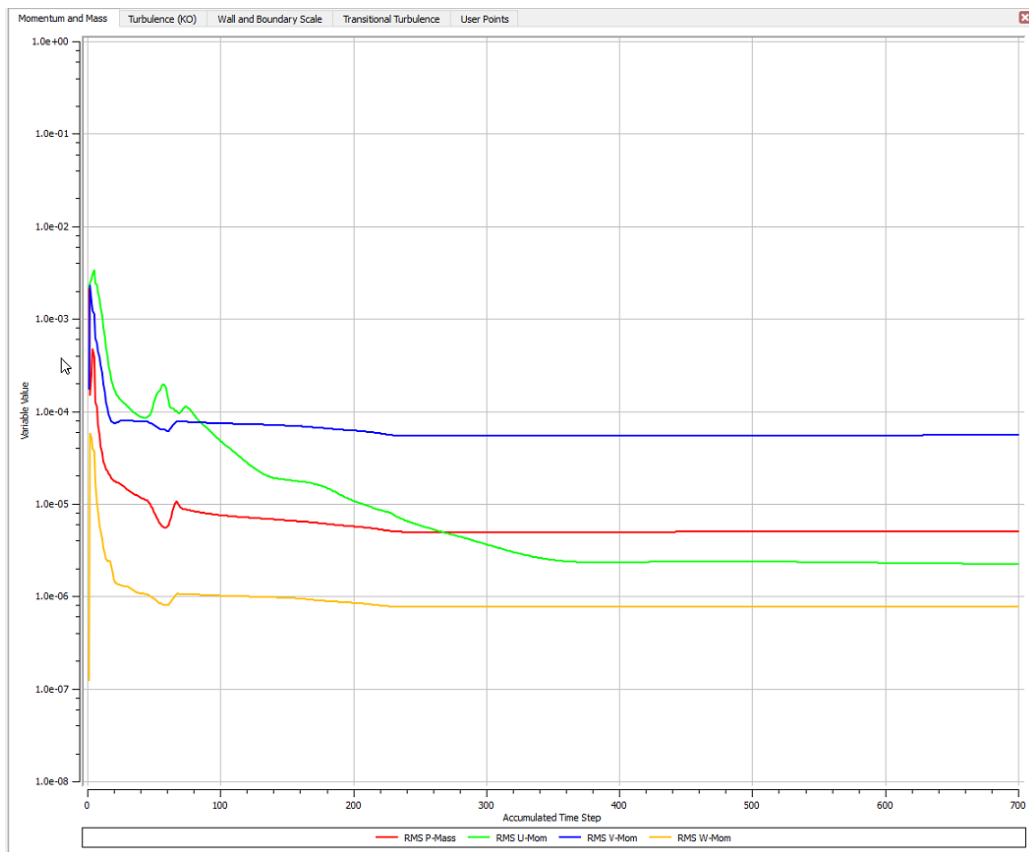
Figure 20. Mass and momentum convergence single element airfoil at AoA 4^\circ Reynolds number 3 million
