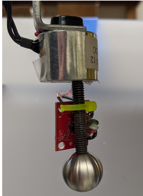
Figure 3.1. Intruder and accelerometer used in impact experiments.
