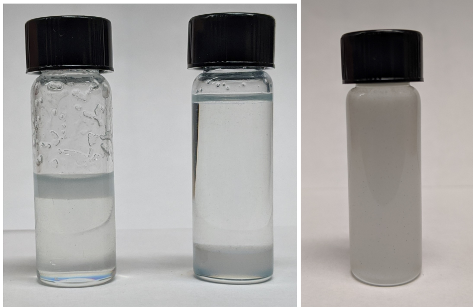
Figure 3.3. Left: Borosilicate microspheres floating in a very dense SPT-water mixture versus microspheres settled in a less dense mixture. Right: A density-matched SPT-water mixture containing soda-lime microspheres.
