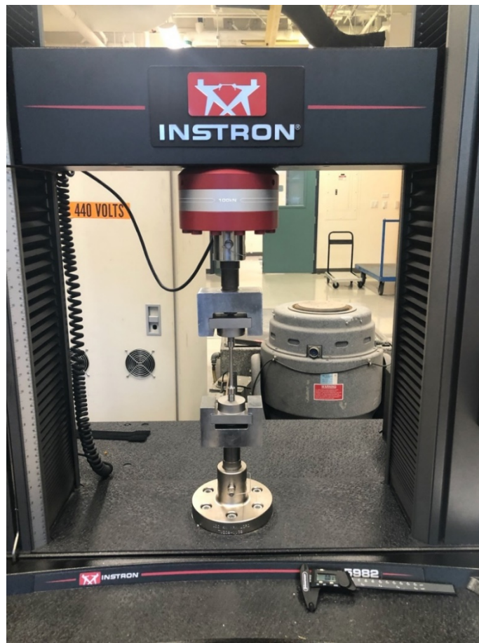
Figure 8. Instron 5982 used to measure tensile properties of parts.
