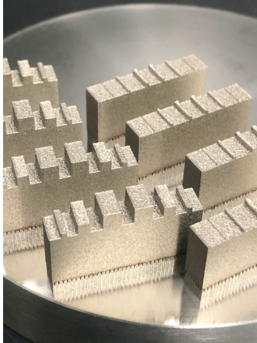
Figure 26. Maraging steel feature size samples printed from EOSM100.
