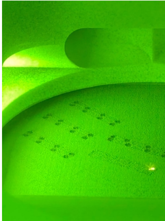
Figure 25. Live imaging of the support structure during printing of maraging steel parts.
