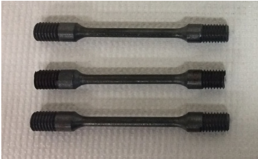
Figure 7. HT tensile test specimens.
