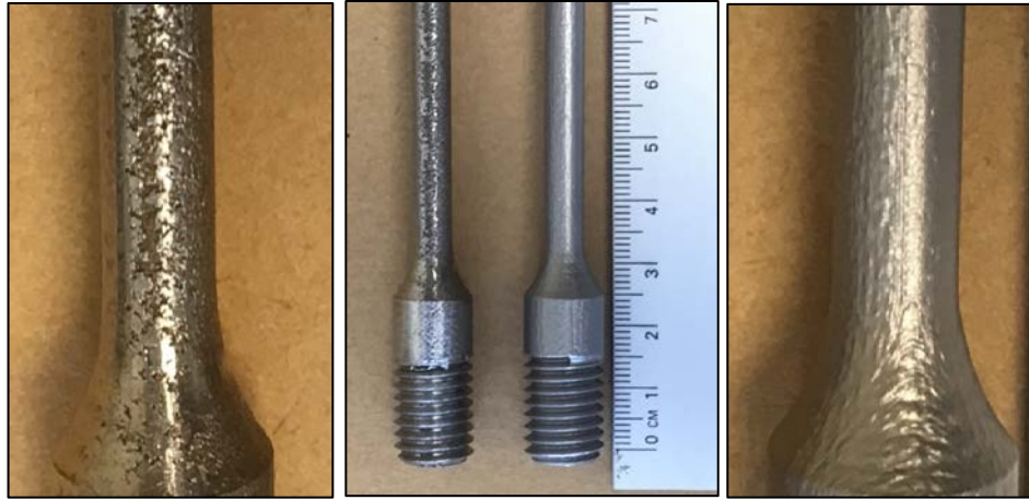
Figure 14. AP versus sandblasted surface.
