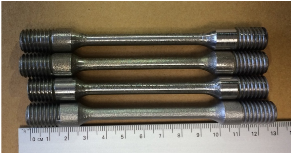
Figure 6. AP tensile test specimens.
