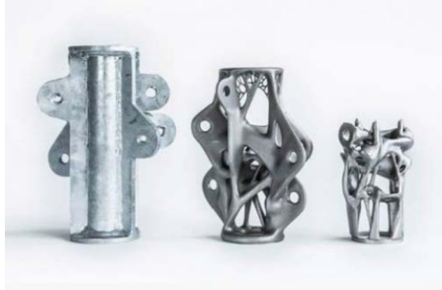
Figure 2. Geometrical complexity of AM versus TM part. Source: [9].
