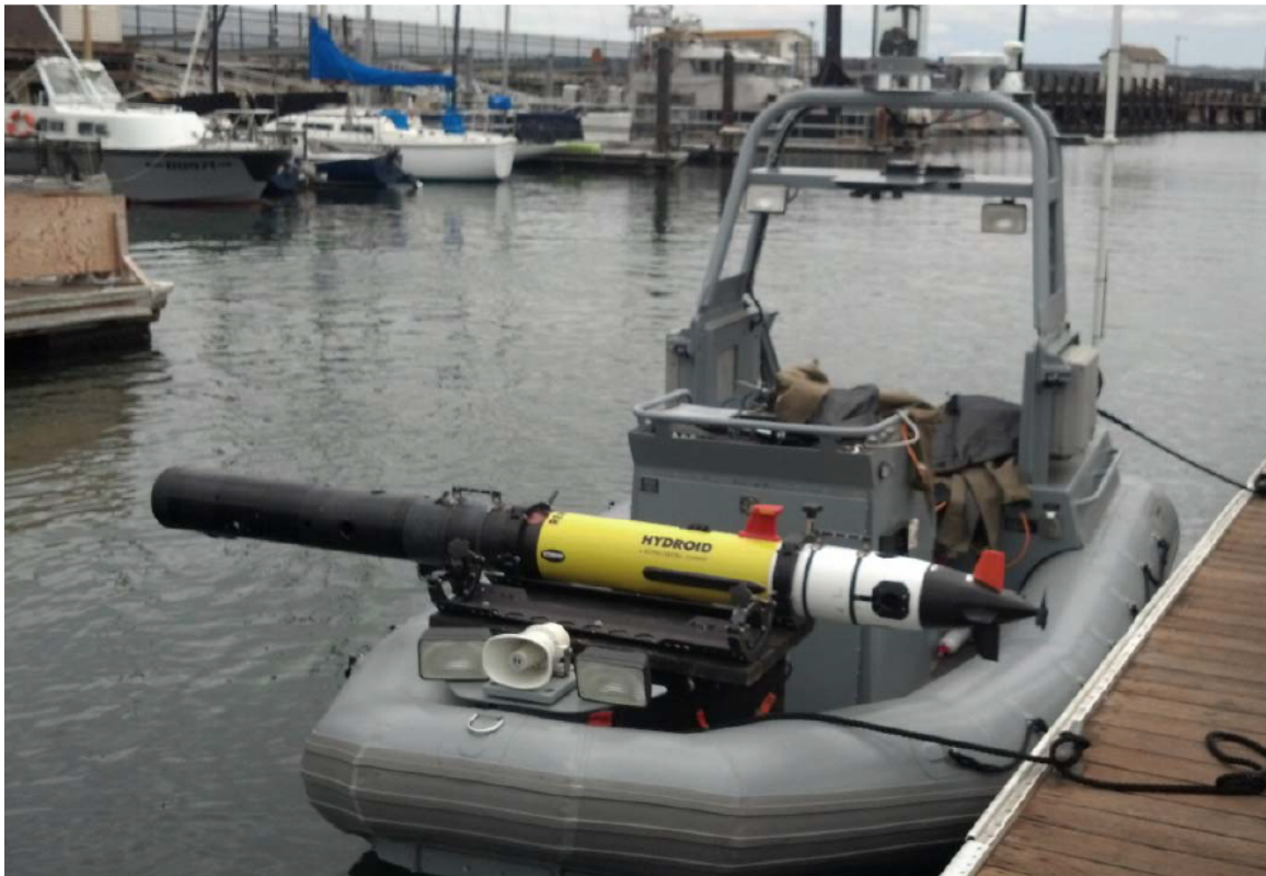
Figure 1.4. REMUS 100 AUV onboard CAVR's SeaFox surface vessel
