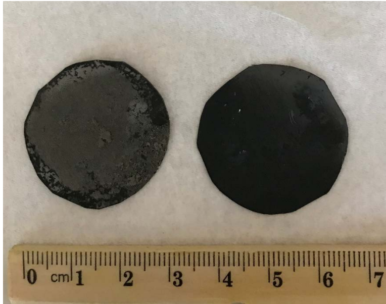
Figure 37. Iron discs with cermet coating (left) and no coating (right).
