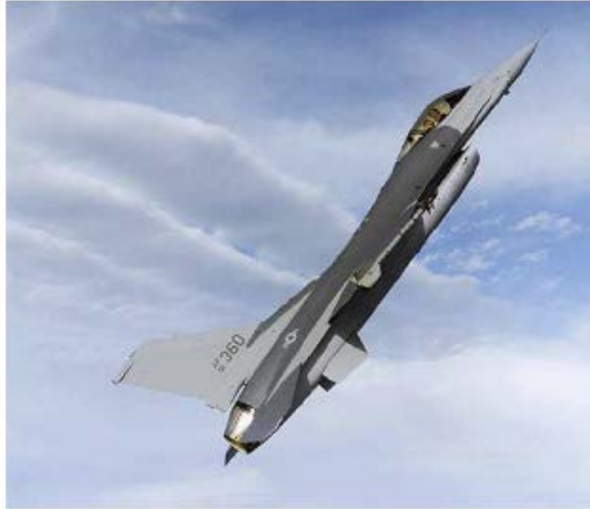
Figure 5. F-16 showing the ventral fin at the back of the aircraft. Source: [8].
