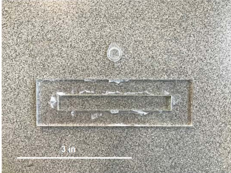
Figure 13. Types of molds used to form the powder mixtures before treatment.
