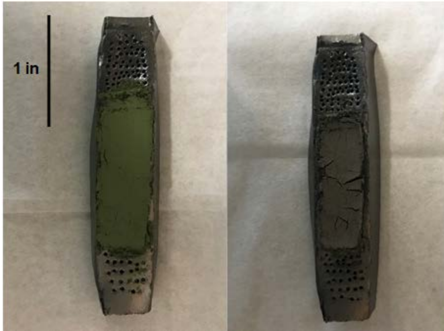
Figure 22. Comparison of a powder pack before and after heat treatment.
