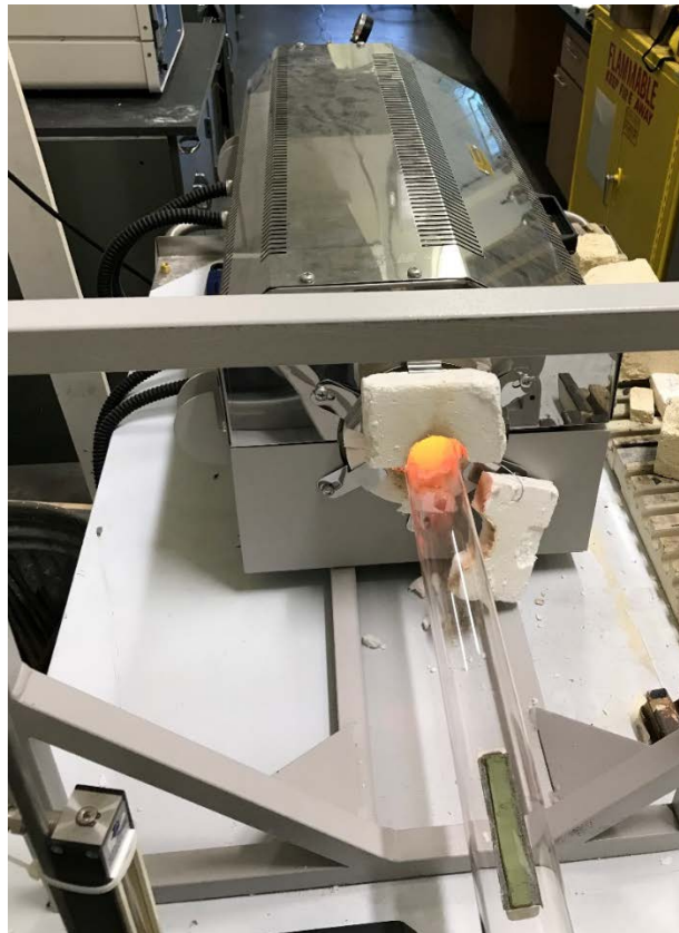
Figure 10. Clam-shell furnace with the molded nickel powder before insertion.
