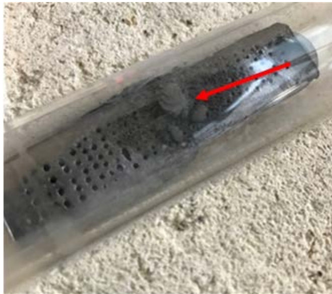
Figure 19. Alumina mixture after heat treatment (blown apart).
