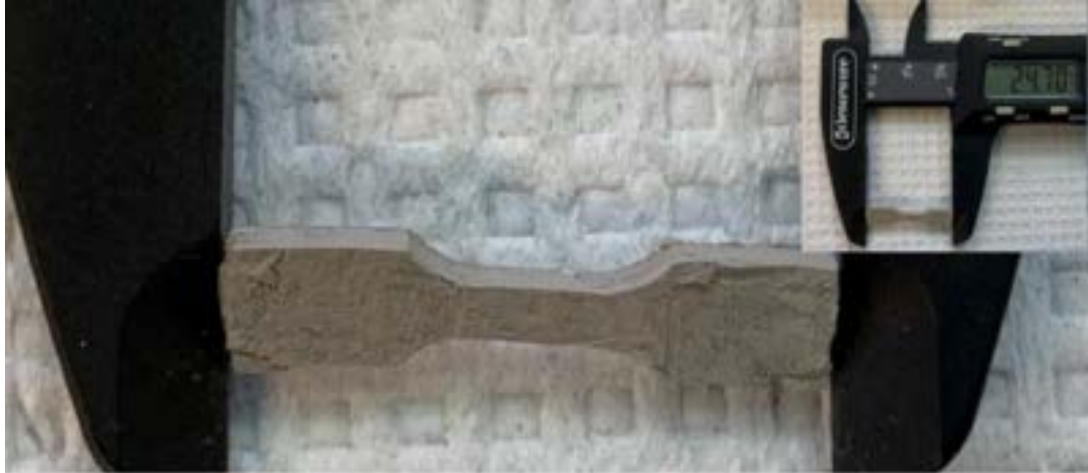
A rectangular nickel body created through RES showing faithfulness to mold shape and indicating significant sintering.
