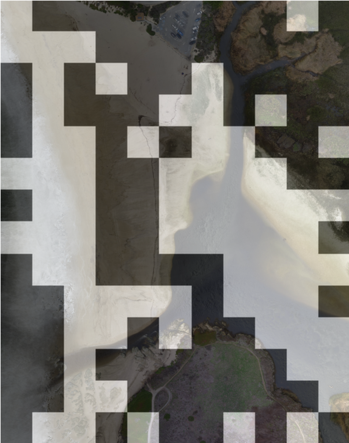
Figure 5.15. Example of VGG19 change detection with 512x512 tiles overlaid on the January orthorectified image.
