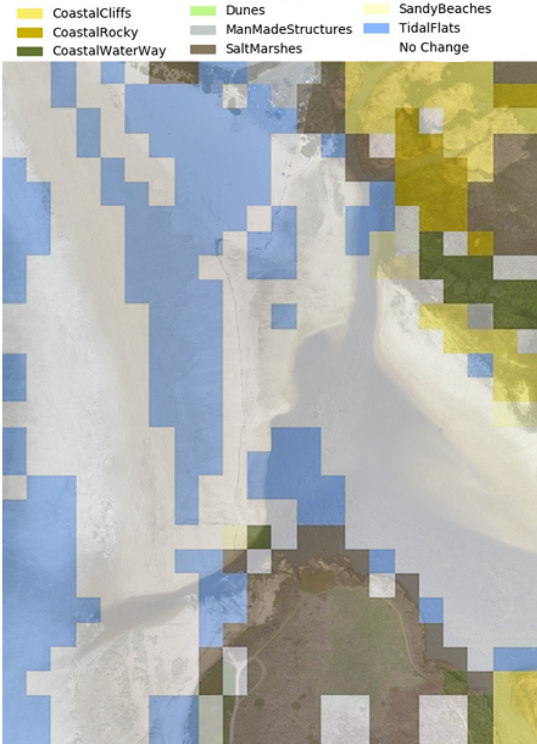
Figure 5.17. January 10, 2018 orthorectified image with 512x512 sliding window pixel tile change detection graphic overlay.
