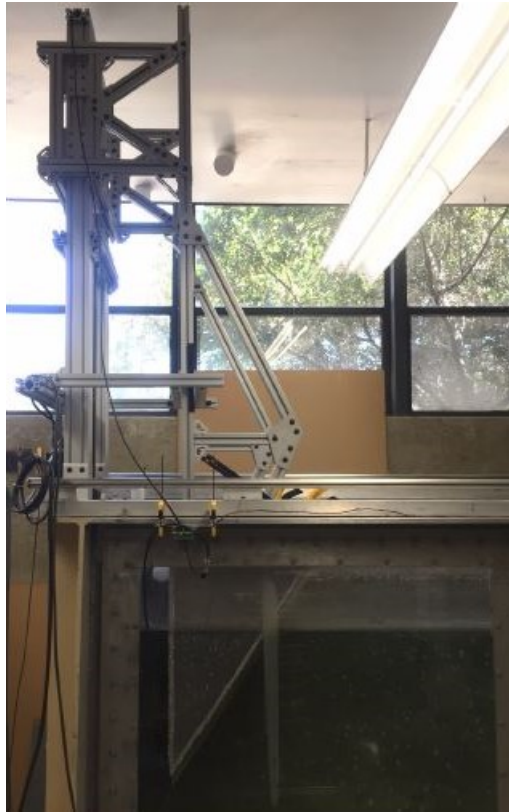
Figure 3.2. Side view of the wavemaker system. Source: [25].
