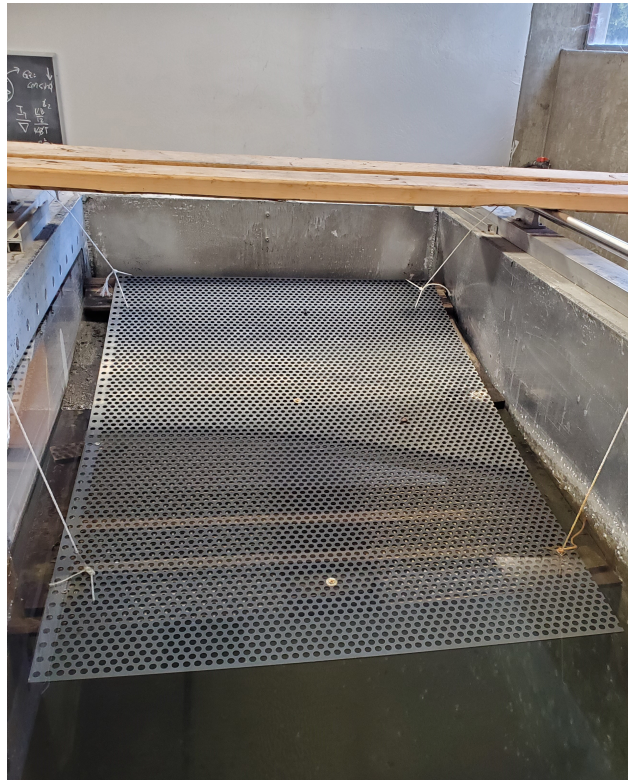
Figure 3.3. Wave-absorbing beach used to reduce the energy of reflected waves.
