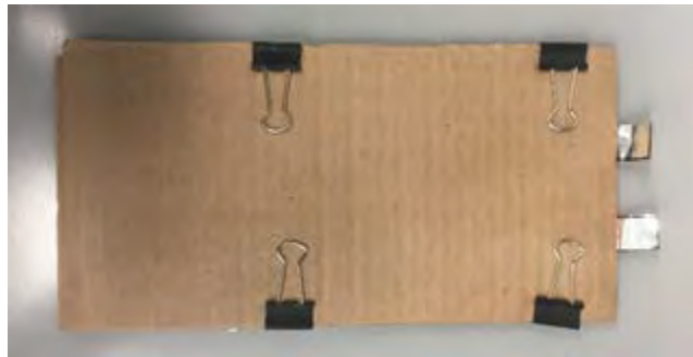
Figure 31. Completed plastic capacitor
