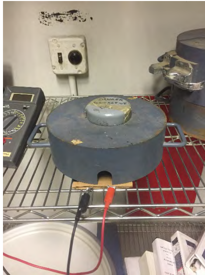
Figure 32. Cs-137 capacitor under lead shield
