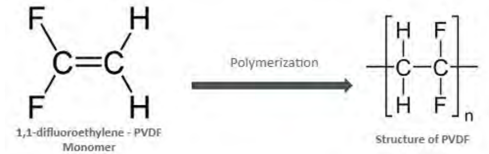
Figure 8. Polymerization of PVDF. Source: [15].
