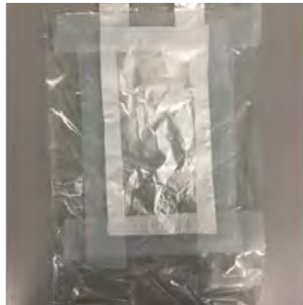
Figure 29. Aluminum foil taped to capacitor
