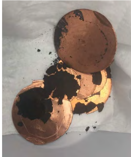
Figure 13. Copper plate capacitor disassembly
