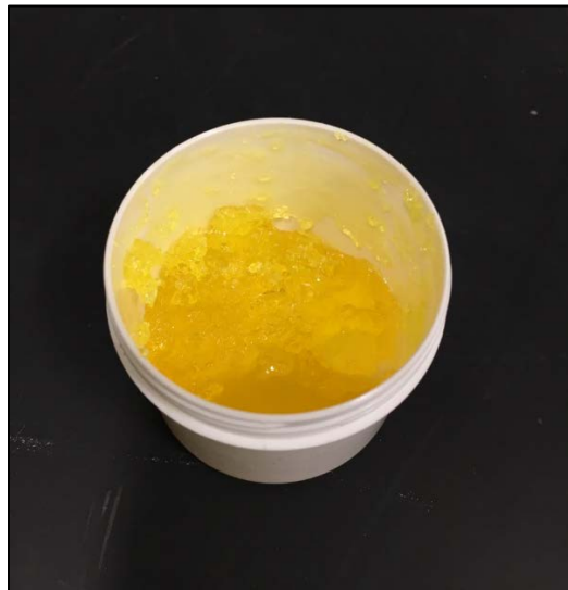
Figure 36. Pre-processed Sample of SMP-10 in 50 mL FlackTek Container
