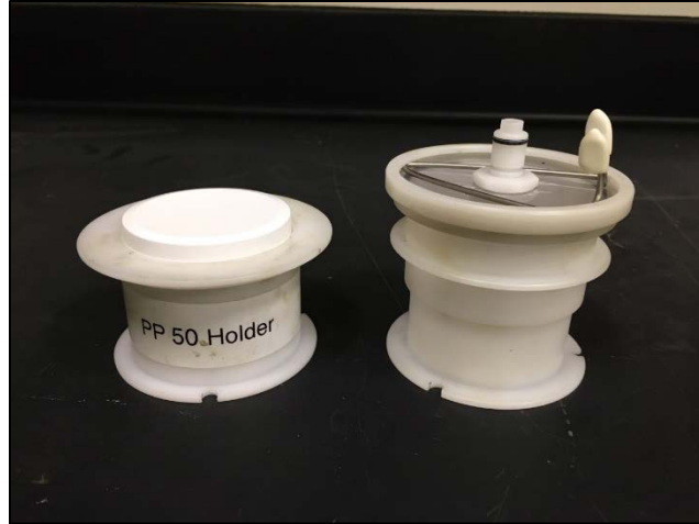
Figure 20. Standard FlackTek 50 mL Container Holder (left) and 50 mL Container Holder for Vacuum Mixing (right)
