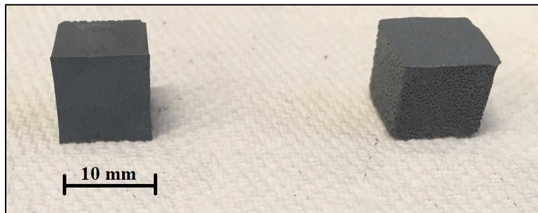
Figure 46. First Full Cure Molded Cubes at 100°C Initial Cure (left) and 130°C Initial Cure (right)
