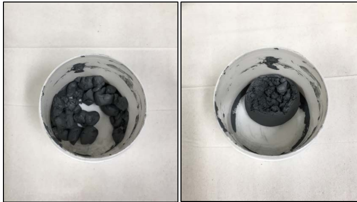
Figure 39. SiC Powder/SMP-10 Mixture after 1,200 RPM (left) and 3,000 RPM (right)
