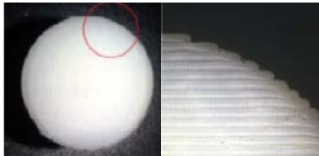
Figure 2. SEM Imaging of Layer-by-Layer Build Part. Source: [13].
