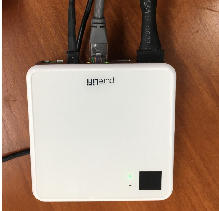
Figure 9. PureLifi access point connected to Ethernet and luminair during an initial test out of the box
