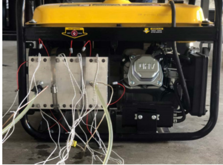
Figure 4. Water-cooled thermoelectric generator waste heat harvesting prototype. Source: [15].
