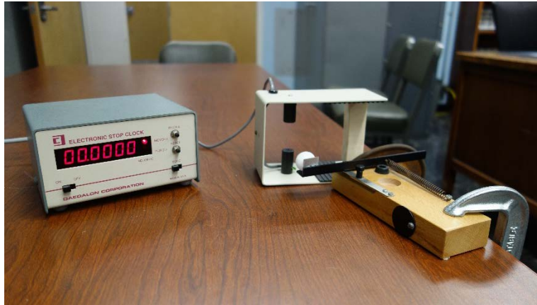
Photogate apparatus with stop clock to measure the initial velocity v_0 of the Styrofoam ball. The diameter is divided by the maximum interrupt time.
