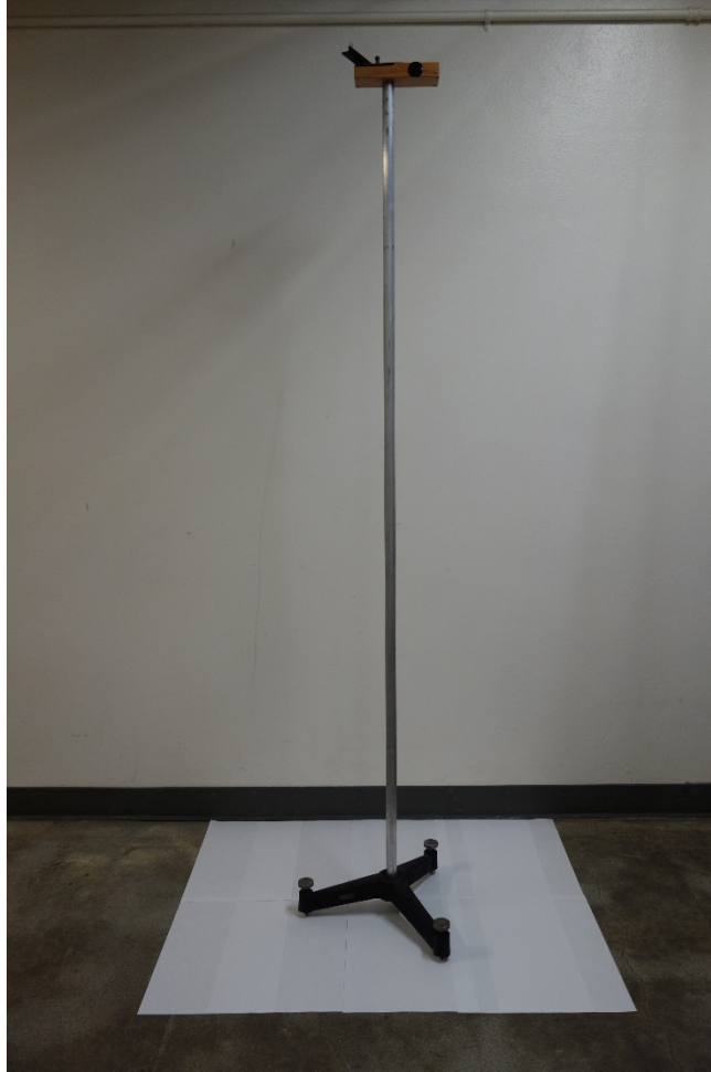
Drop-launch mechanism mounted on a large modified tripod. The height of the entire apparatus is nearly 2 m.
