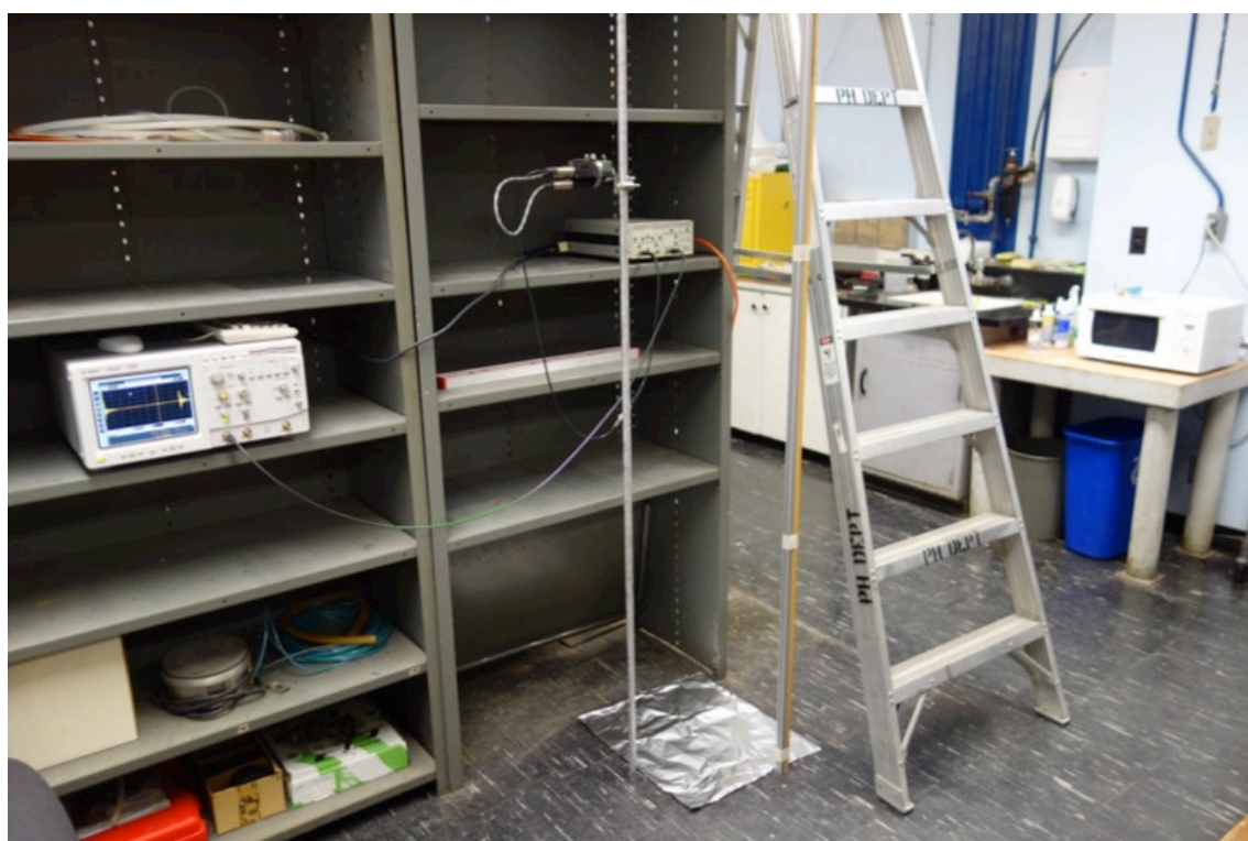
Figure 9. Upper and Lower Parts of Apparatus to Determine the Drag Coefficient of a Styrofoam Ball.
