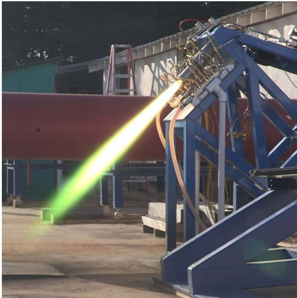
Figure 50. Changing Exhaust Color Indicating Component Failure During Nov21Run01
