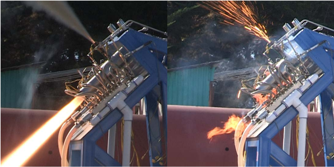
Figure 54. Ignitor Failure During Nov12Run03
