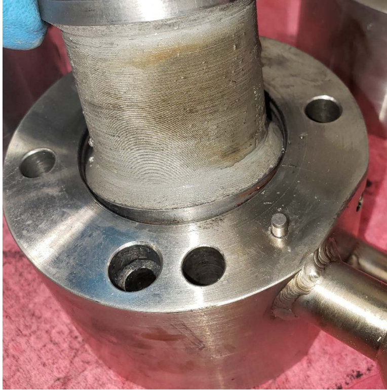
Figure 39. Spool Discoloration After Apr09Run03
