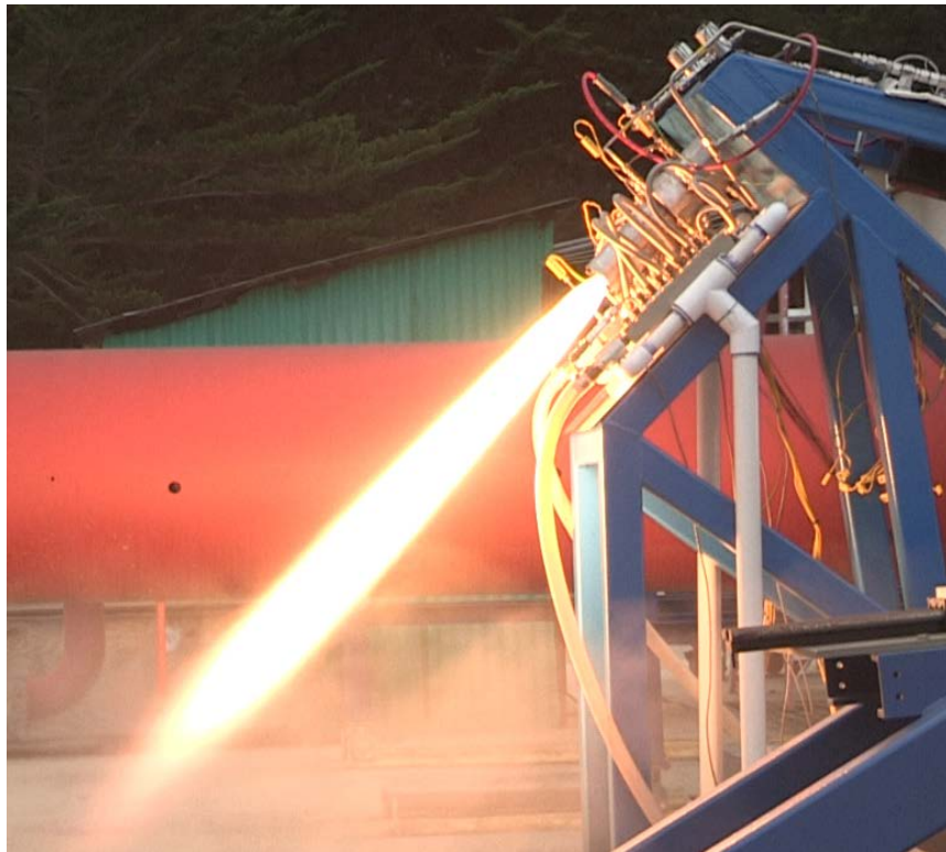
Figure 18. Main Camera View of a Nominal Engine Run
