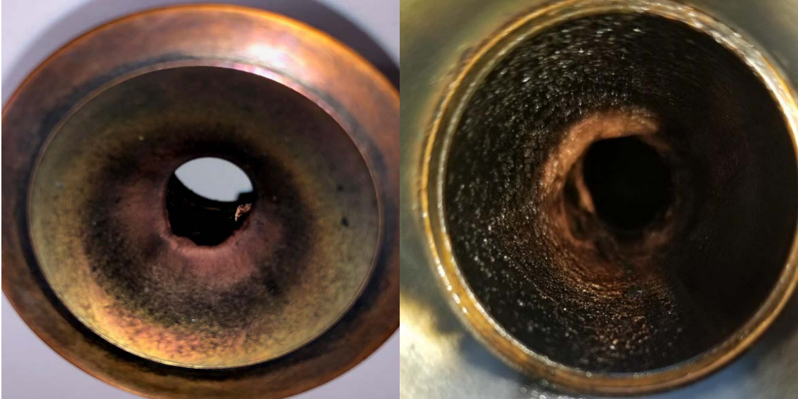
Figure 51. Failed 1.27 cm Nozzle Converging and Diverging Sections
