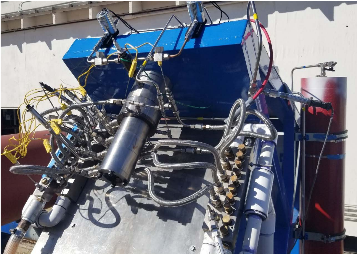
Figure 12. Liquid Rocket Engine Mounted on Test Stand
