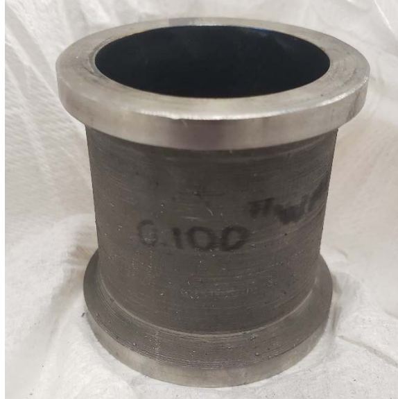
Figure 41. 0.254 cm Spool After Pressure Test
