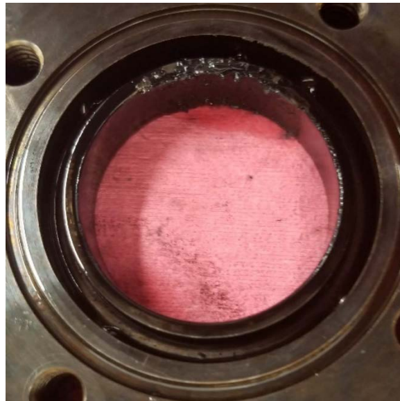
Figure 52. Failed Film Cooling Ring
