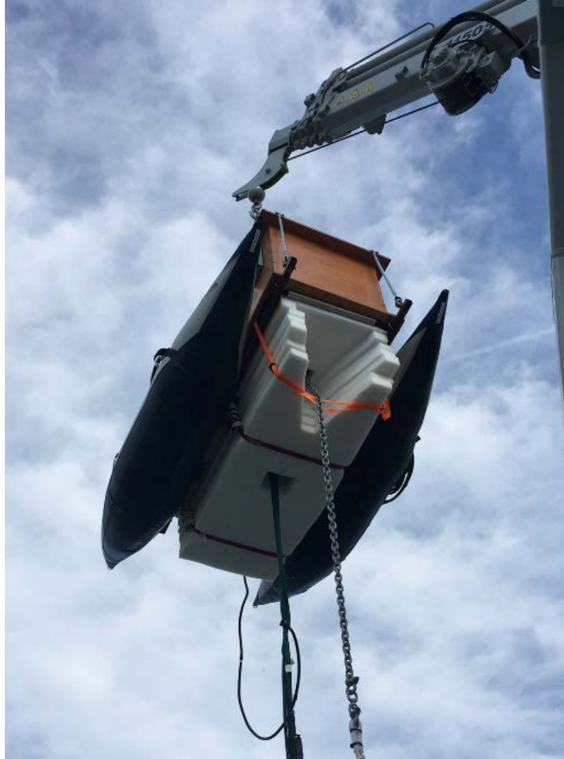
The underside of the “coffin” (hanging from the ship’s crane) showing the additional floatation, the anchor chain/line and the line from which the acoustic source was suspended.
