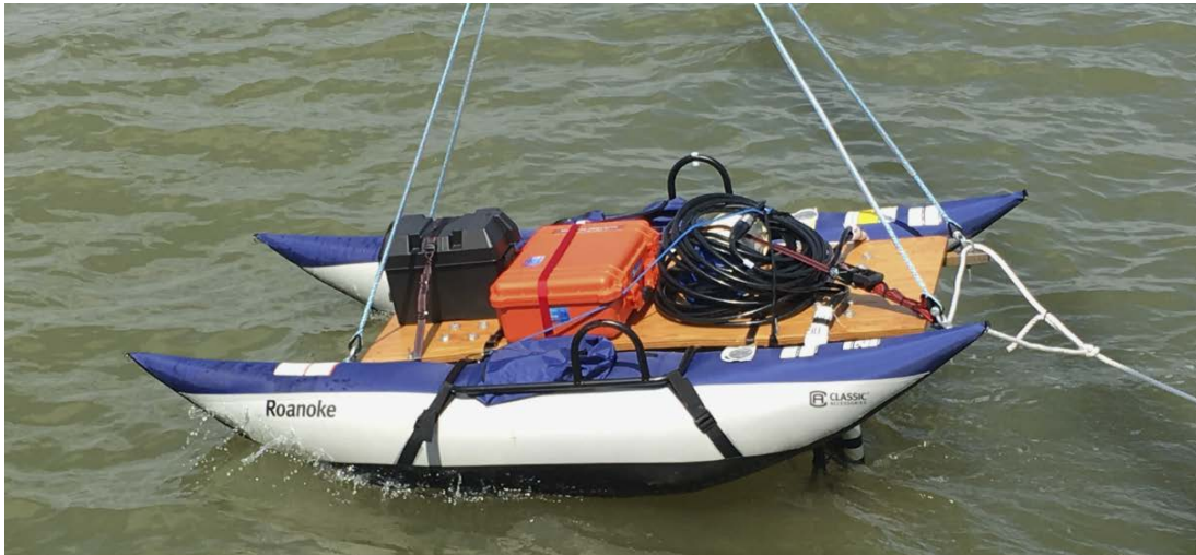
The Banshee deployed from the ship's crane alongside the R/V Virginia on 24 April 2019. The 12 vdc marine battery is in the black box on the left, the BioSonics electronics is housed in the orange watertight case and the excess cable is secured on the right.
