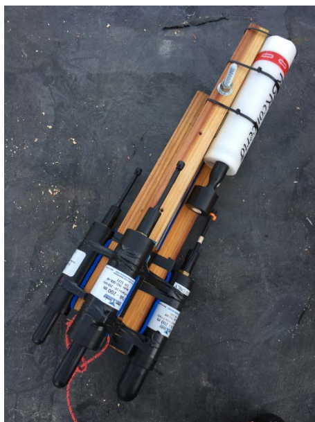
The bubble device was deployed over the side of R/V Virginia on 24 April 2019 during the same period that the Banshee was in the water. The CTD is the white cylinder at the top of the picture and the two acoustic projectors and hydrophone are attached to the bottom of the wooden frame.
