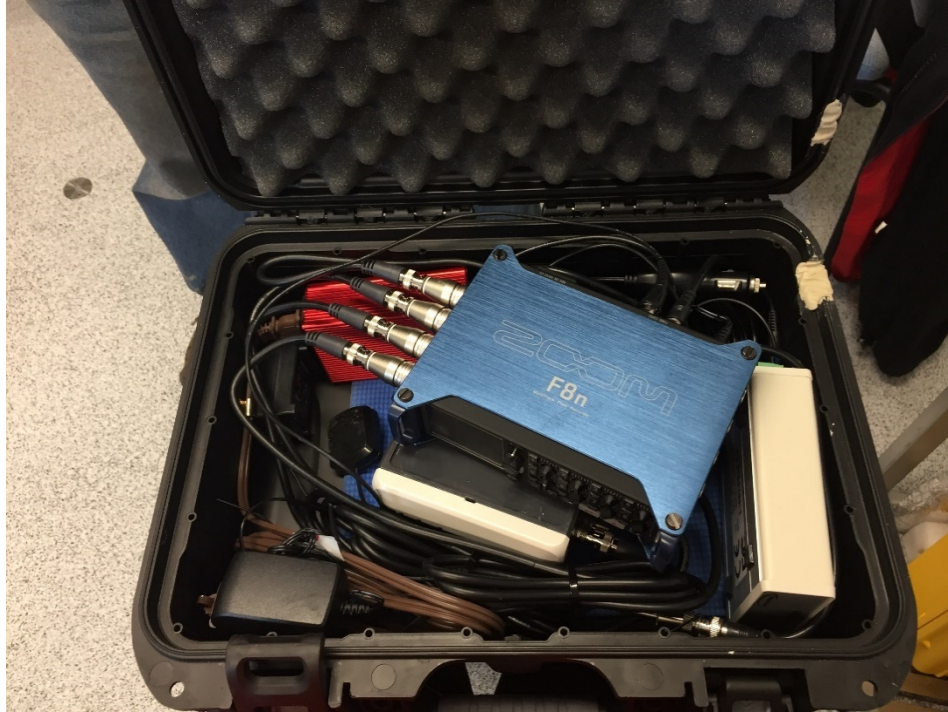
The electronics inside the watertight case shown on the mini-cat in Figure 10. The case contained the Zoom F8n 8-channel recorder (blue), the 8-channel pre-amp (gray/white), the GPS time-code generator (cream) and the 12v inverter (red).
