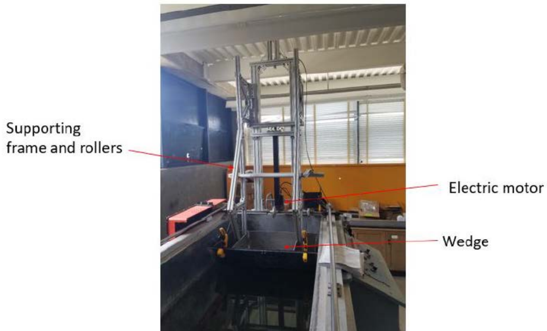
Figure 4. NPS tow tank wave generation assembly. Source: [9].
