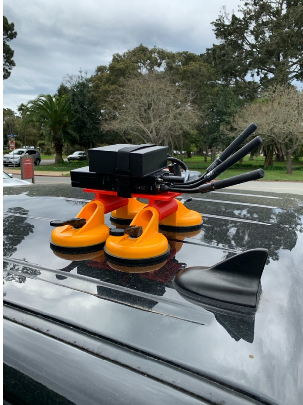
Figure 38. Hypernode Mounted to Roof of Author's Truck
