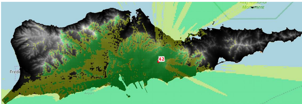
Figure 4.5. Coverage Map of Tower 42 on St. Croix. While tower 42 appears centrally located, nearby topography leads to high losses. Thus, the tower provides only medium coverage for nearby populated areas. White/grayscale/black represents elevation, yellow represents medium coverage, and green represents good coverage.
