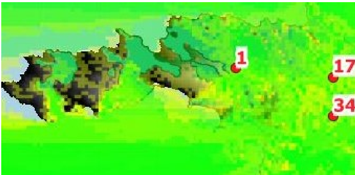
Figure 4.9. Coverage Map of Western STT Compared with VI Coverage PowerNet from 2014. Coverage in western STT aligns to the VI PowerNet data. Notice coverage gaps directly west of Tower 1. In this area, cellular service only seems to exist on the hilltops, while service is lost in the valleys and on the coast. White/grayscale/black represents elevation, yellow represents medium coverage, green represents good coverage, and teal is VI PowerNet coverage from 2014.
