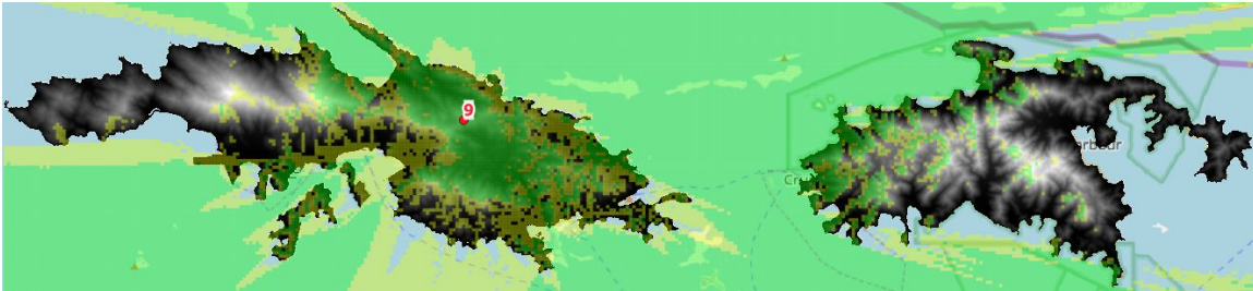
Figure 4.13. Coverage Map of Tower 9 on St. Thomas. Tower 9 is located on a high elevation point in northwestern STT. From here, it provides equal amounts of good and medium coverage across both STT and STJ. White/grayscale/black represents elevation, yellow represents medium coverage, and green represents good coverage.
