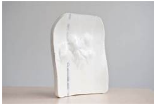
Figure 1. Image of a pressed UHMWPE textile armor backing system.
