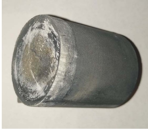
Figure 29. Sample could not be separated from the punch.
