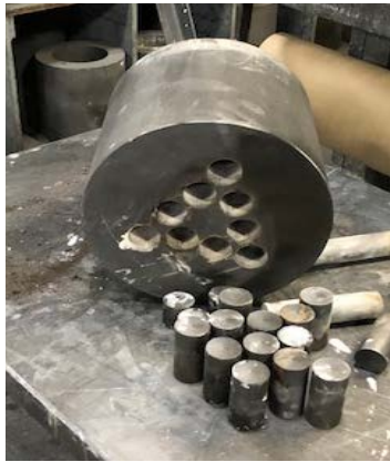
Figure 28. A bench view of the die, punches, and powders post-heating and pressing.
