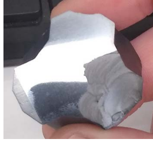
Figure 33. Damaged test sample with high polish.
