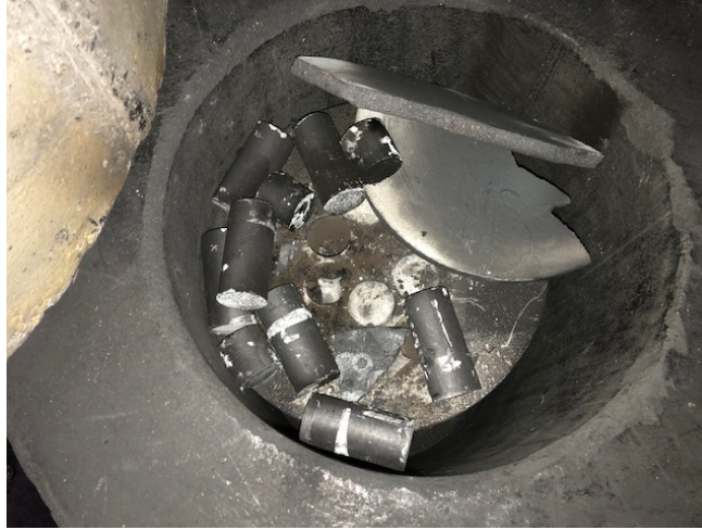
Figure 31. Damage caused by the 5 atom alloyed powder.
