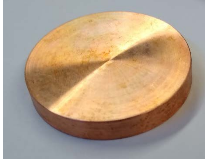
Figure 54. 38mm diameter Cu impactor.
