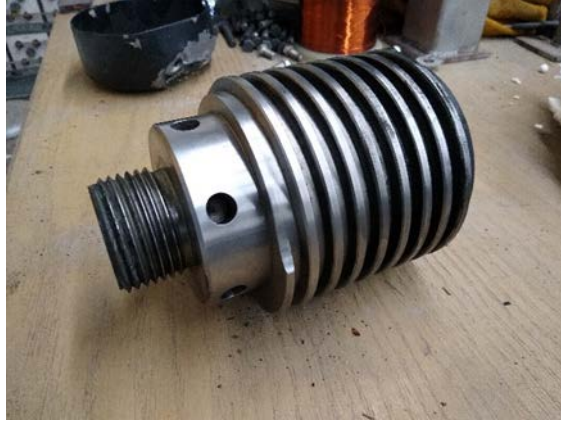
Figure 46. The breach plug securely constrains the main charge, holds the secondary charge, and attaches the firing solenoid.
