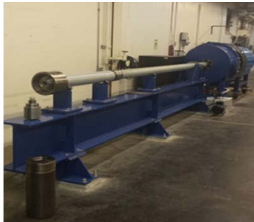
Figure 43. 40mm single-stage powder gun.
