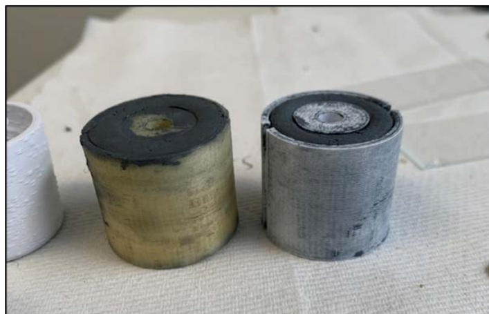
Figure 59. Molded, SiC Rocket Nozzle (One Water-Soluble Mold-Left and One PLA Mold-Right) Side View.
