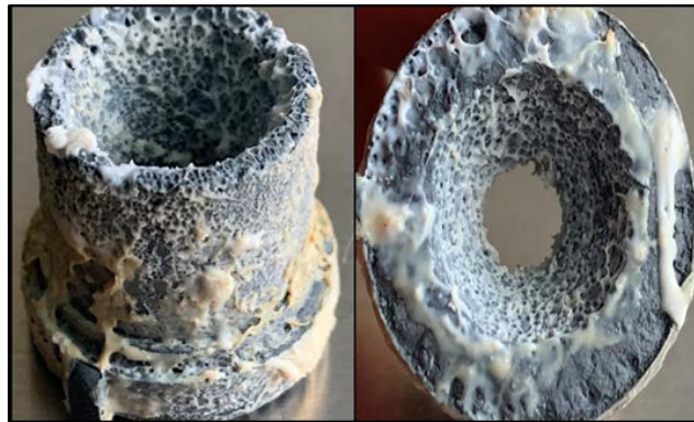
Figure 61. Post-Cured Rocket Nozzle with Remnants of PLA Mold Melted on SiC.
