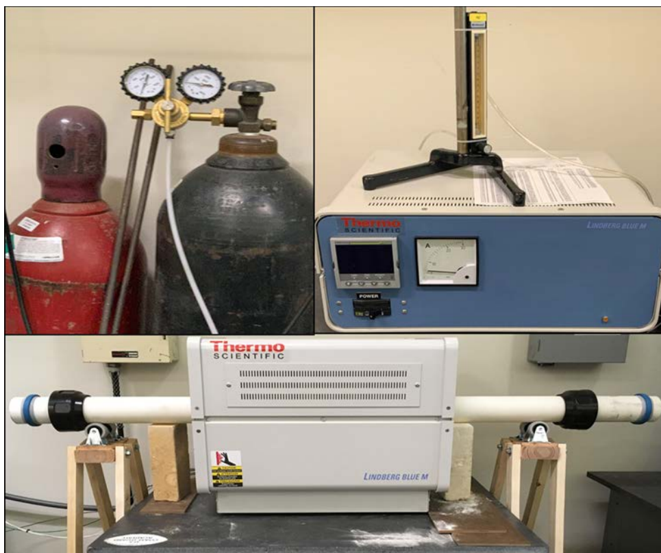
Figure 20. Gas Tanks Pictured in Top Left (Connected to Nitrogen-Green Tank), Control Module in Top Right, and Tube Furnace in Bottom Center with Partial Endcaps on Tube (Denoted Black).
