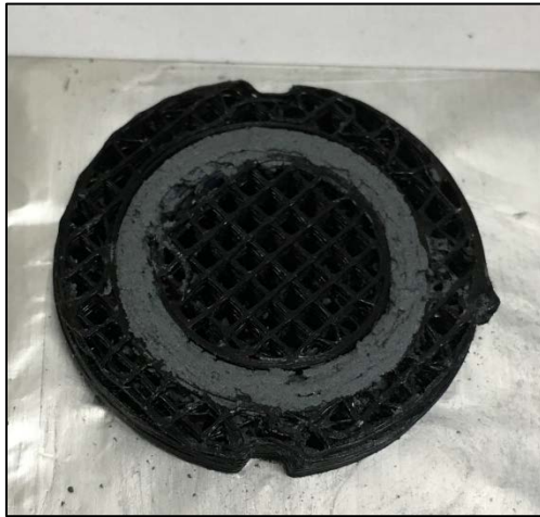
Figure 69. Dual-Extrusion, VAP, Partial Rocket Nozzle Trial with SiC Polymer Infill.
