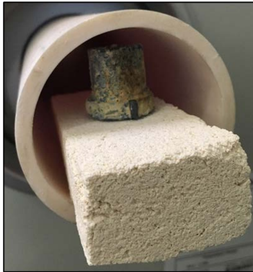
Figure 63. Post-Cured Rocket Nozzle (from Figure 61) Being Placed in Furnace for Setup of Pyrolysis.
