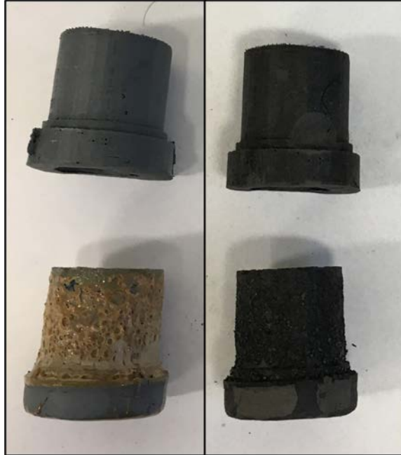
Figure 65. PVA (Top) vs. PLA (Bottom) Rocket Nozzle Pre-Pyrolysis (Left) vs. Post-Pyrolysis (Right) Trial.
