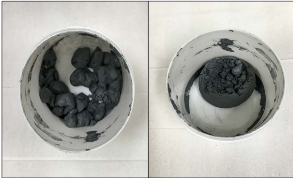
Figure 16. SiC Powder + SMP-10 Mixture (Left-After Mixing at 1200 RPM, Right-After Mixing at 3000 RPM).
