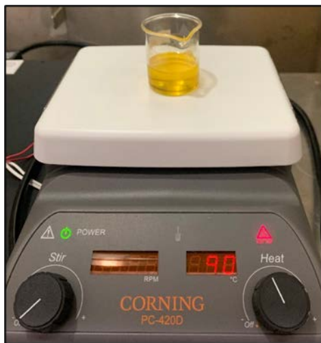
Figure 13. Hot Plate Used for Heating SiC Precursor for Mass Loss.
