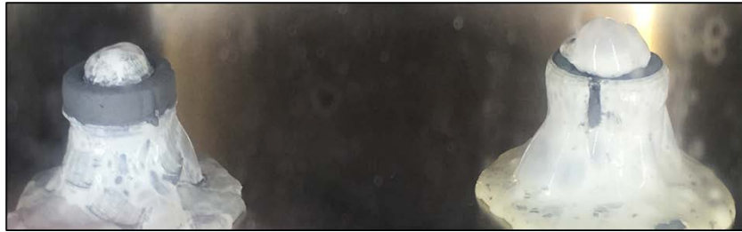
Figure 60. Molten PLA During Curing in Thermovac.
