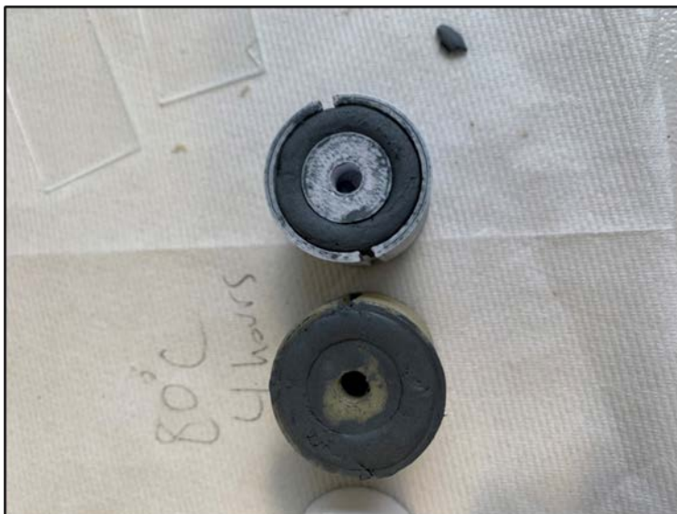
Figure 58. Molded, SiC Rocket Nozzle (One PLA Mold-Top and One Water-Soluble Mold-Bottom) Top View.
