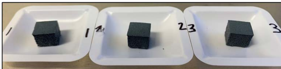
Figure 30. Molded SiC Post-Curing with 50:50 Coarse-to-Fine Powder and 82% Powder and 18% SMP-10 (All 3).
