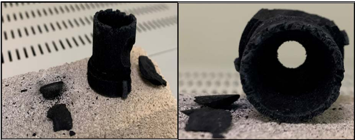
Figure 64. Post-Pyrolyzed Molded Rocket Nozzle from Figure 63.
