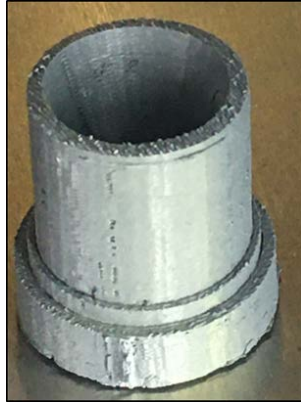
Figure 62. Post-Cured, Rocket Nozzle Mold that was from Water-Soluble Mold.
