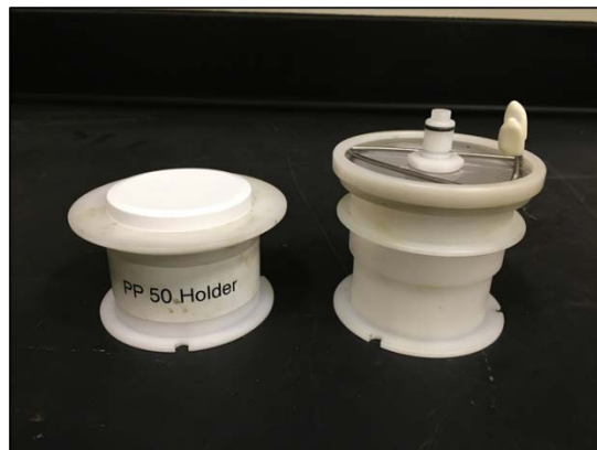
Figure 17. Vacuum-Sealed Holder for SiC + SMP-10 Mixture to be Mixed in.
