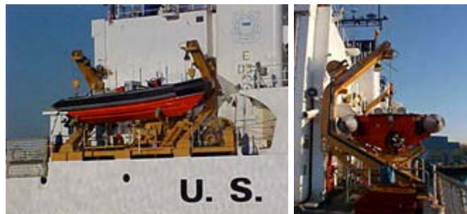
Figure 1. Welin Lambie Dual-Point Davit on a 270-foot MEC, Shown with Cutter Boat Cradled. Source: Welin Lambie (n.d.).
